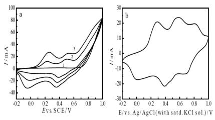
Fig. 1 (a) CVs of the electrochemical synthesis of the polyaniline film on graphite obtained in a solution containing 0.2 M aniline and 0.6 M H<sub>2</sub>SO<sub>4</sub>; (b) the CV of the polyaniline film in a 0.2 M H<sub>2</sub>SO<sub>4</sub> solution at a scan rate of 60 mV s<sup>-1</sup>.
