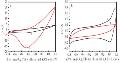
Fig. 4 The CVs of different types of electrodes at a scan rate of 60 mV s<sup>-1</sup>. (a) Curve 1: nano-PAn/N-graphite electrode in CO<sub>2</sub>-saturated water and curve 2: nano-PAn/T-graphite electrode in CO<sub>2</sub>-saturated water; (b) curve 1: nano-PAn/T-graphite electrode in a H<sub>2</sub>SO<sub>4</sub> solution of pH 3.8 and curve 2: nano-T-graphite electrode in CO2-saturated water.
