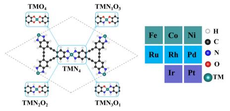
Fig. 1 Optimized geometric configurations of 2D TMN<sub>x</sub>O<sub>4-x</sub>-HTC (x = 0-4) and the considered dopant transition metal atoms.
