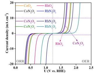
Fig. 6 Simulated polarization curves for the screened-out catalysts.
