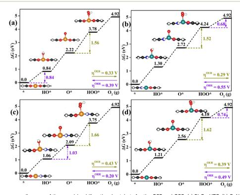
Fig. 4 Calculated free energy diagrams of the promising bifunctional catalysts for the OER and ORR: (a)  $RhO_4$ -HTC, (b)  $CoN_3O_1$ -HTC, (c)  $RhN_2O_2$ -HTC and (d)  $CoN_1O_3$ -HTC. The yellow and pink values are the potential-determining step values for the OER and ORR. The optimized configurations of intermediates on the catalysts are also exhibited.
