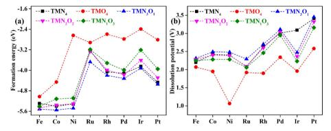
Fig. 2 Calculated (a) formation energy and (b) dissolution potential of transition metal atoms for the designed TMN<sub>x</sub>O<sub>4-x</sub>-HTC catalysts.
