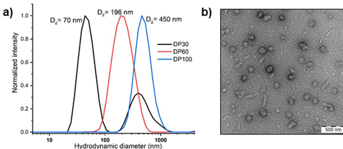
Fig. 6 (a) Hydrodynamic size distributions of PEG<sub>45</sub>-PMTMeOx<sub>x</sub> micelles of different PMTMeOx DP measured by DLS in water ( $c_{\text{pol}} = 1 \text{ mg mL}^{-1}$ ) and (b) TEM image of PEG<sub>45</sub>-*b*-PMTMeOx<sub>30</sub> nanoparticles.
