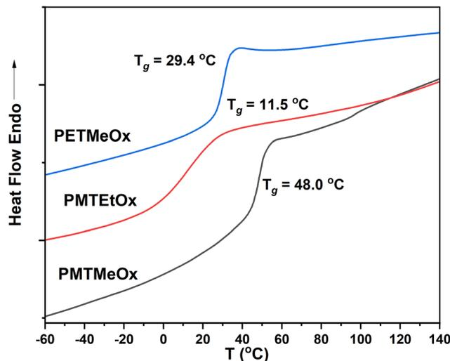
Fig. 3 DSC curves of the homopolymers.
