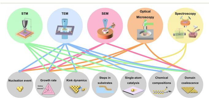
Fig. 1 Schematic illustration of the used in situ techniques for 2D materials growth and the related research on the growth dynamics.
