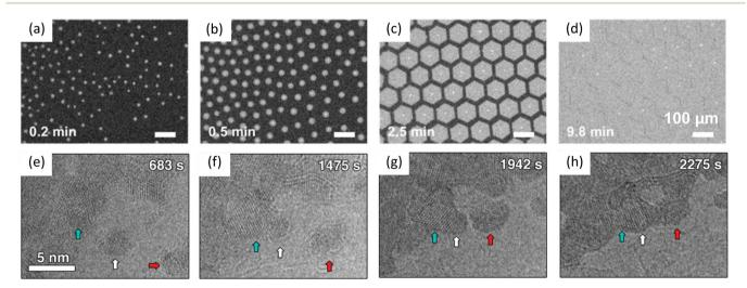
Fig. 6 Schematic illustration of in situ imaging of domain coalescence processes during graphene growth and MoS2 growth. (a-d) In situ optical imaging of graphene growth on liquid copper. Reproduced from ref. 62 with permission from American Chemical Society, copyright 2021. (e-h) TEM images showing coalescence of MoS<sub>2</sub> grains. Grains indicated by white and red arrows move toward the grain indicated by cyan arrow. Reproduced from ref. 88 with permission from Wiley, copyright 2019.
