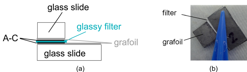
Fig. 2 (a) A cross section of the sample with grafoil coated active carbon (AC) electrodes and (b) a picture of the cover area ca. 1.27 \times 1.27 \text{ cm}^2 .
