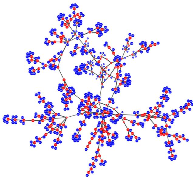
**Fig. 1** Graph representation of a network of inherent structures of a glassy atactic polystyrene specimen at room temperature ( $T = 300$  K) and atmospheric pressure. Red nodes denote “explored” while blue ones denote “boundary” states. The snapshot has been created at the very early stages of the network expansion.
