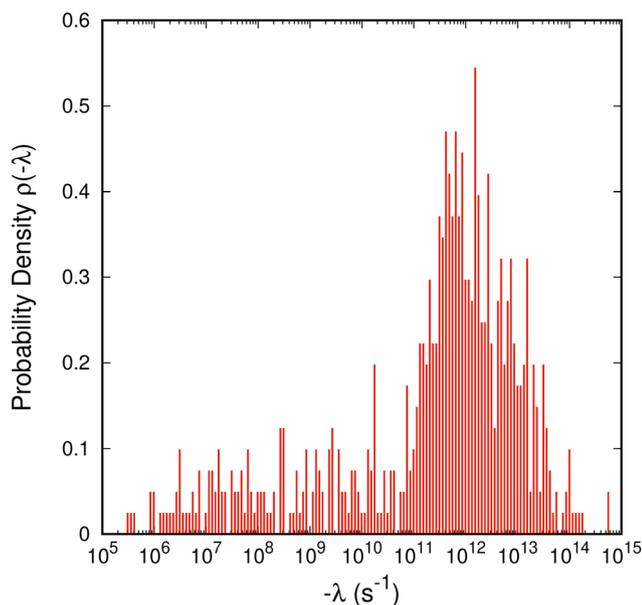
**Fig. 4** Histogram of the characteristic rates (negative eigenvalues) of the rate constant matrix,  $K$ , governing the dynamical evolution of a network of states (eqn (2)) of aPS at  $T = 300$  K. The bins are equally spaced on the logarithmic axis and the distribution is normalised such that  $\int \rho(-\lambda) d \log_{10}(-\lambda/s^{-1}) = 1$  holds.
