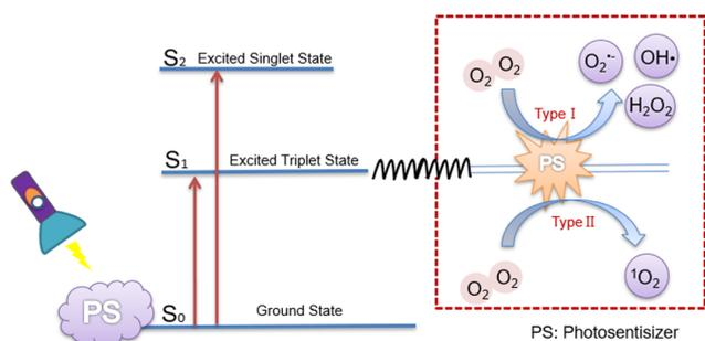
Fig. 1 Two types of mechanism of ROS generation by photosensitizers.<sup>14</sup>
