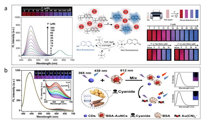
Fig. 7 (a) Detection of fluoride by the use of ratiometric sensing. 116 Adapted with permission from ref. 116. Copyright 2017. Royal Society of Chemistry. (b) Detection of cyanide by the use of ratiometric sensing. Adapted with permission from ref. 102. Copyright 2019. Springer Nature.
