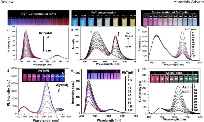
Fig. 5 Ratiometric detection of different metals by quantum dots and other fluorescent materials (a) mercury<sup>101</sup> (b) iron<sup>109</sup> (c) copper<sup>78</sup> (d) silver<sup>79</sup> (e) lead 112 (f) arsenic. 80 Reproduced with permission from ref. 101, 109, 78, 79, 112 and 80. Copyright 2018, 2016, 2016, 2020, 2019, 2016. Royal Society of Chemistry, Royal Society of Chemistry, Royal Society of Chemistry, Springer Nature, American Chemical Society, American Chemical Society.
