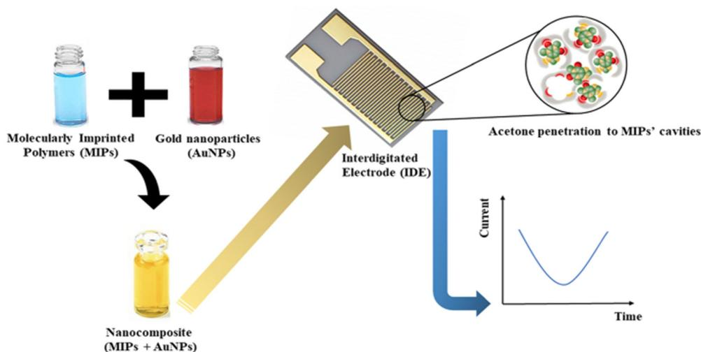
Fig. 11 Diagrammatic illustration of MIP@Au nanosensors for the detection of acetone gas.<sup>64</sup> Copyright©2022, Iran Polymer and Petrochemical Institute.
