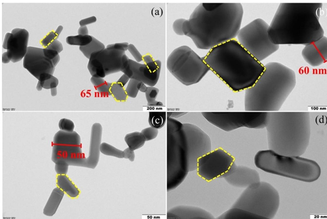
Fig. 9 (a)–(d) HRTEM images of ZnO NPs in the 200, 100, 50, and 20 nm scale range.<sup>57</sup> Copyright ©2022 Elsevier B.V. All rights reserved.
