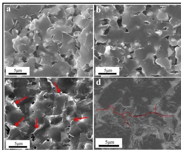
Fig. 15 Fracture surfaces of hot-press sintered  $B_4C$ -20 wt% SiC ceramics produced at different sintering pressures: (a) 30 MPa, (b) 35 MPa, and (c) 40 MPa.<sup>122</sup> (d) Indentation crack deflection in hot-press sintered  $B_4C$ -20 wt% SiC ceramics produced at a sintering pressure of 40 MPa.<sup>122</sup>
