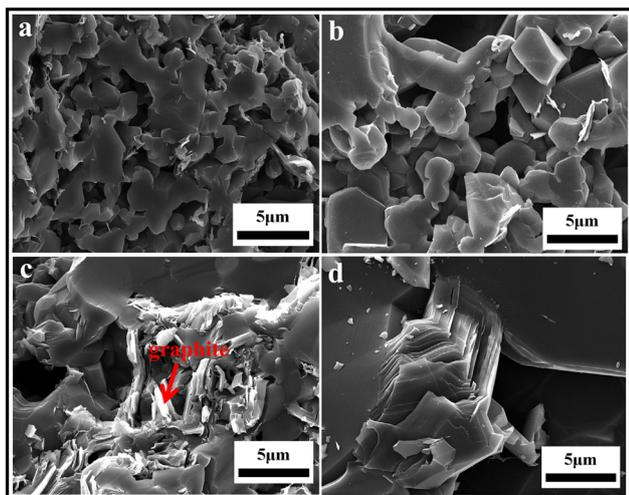
Fig. 5 Fracture surfaces of pressureless sintered  $B_4C$ -15 wt% SiC ceramics sintered at: (a) 2100 °C, (b) 2125 °C, (c) 2150 °C, and (d) 2175 °C<sup>107</sup> (reprinted with permission, Copyright 2019, Elsevier).
