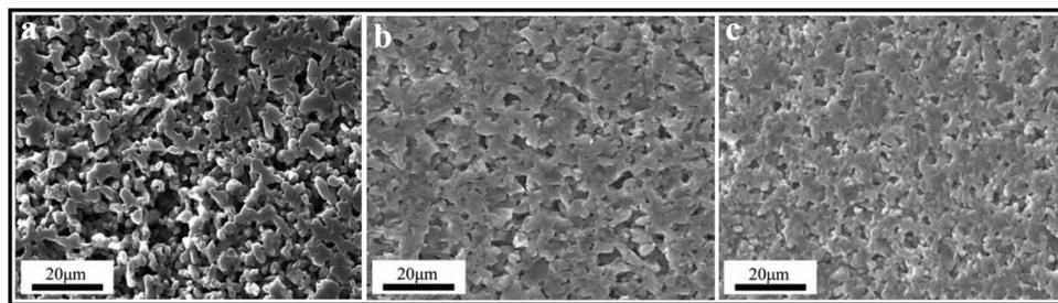
Fig. 6 Microstructure of hot-press sintered B<sub>4</sub>C–20 wt% SiC ceramics sintered under different sintering pressures: (a) 30 MPa, (b) 35 MPa, and (c) 40 MPa.<sup>122</sup>
