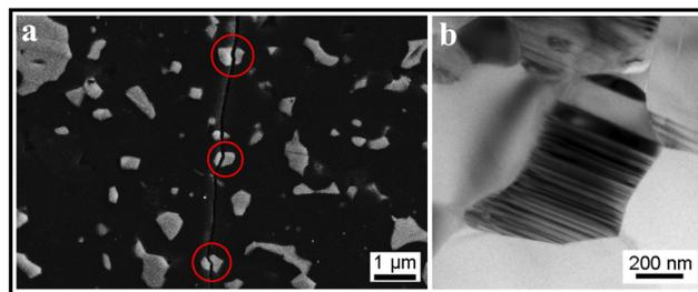
Fig. 12 (a) Cracks in spark plasma sintered B<sub>4</sub>C–SiC ceramics whose SiC is generated from PCS pyrolysis showing frequent deflection and (b) SiC grain generated from PCS pyrolysis in the B<sub>4</sub>C–SiC ceramics showing a layered structure (or planar defects)<sup>87</sup> (reprinted with permission, Copyright 2018, Elsevier).
