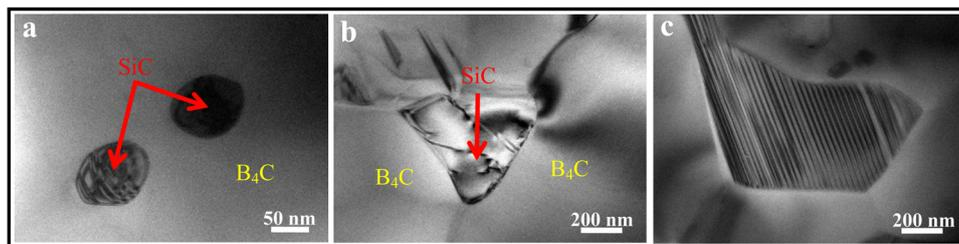
Fig. 3 TEM images of hot-press sintered  $B_4C$ -15 wt% SiC ceramics produced *via* the introduction of SiC in the form of PCS: (a) intragranular SiC structure, (b) intergranular SiC structure, and (c) SiC grains with a layered structure<sup>91</sup> (reproduced with permission, Copyright 2013, Elsevier).
