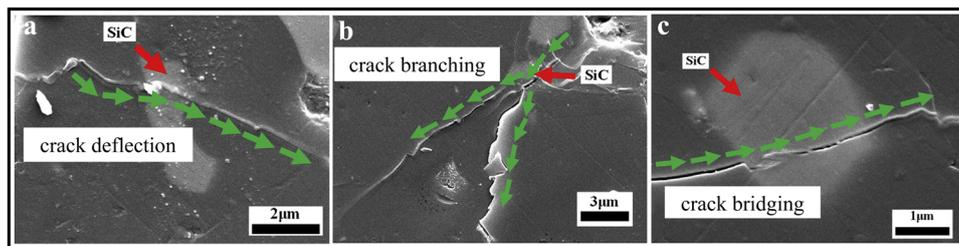
Fig. 13 Crack propagation on the surface of pressureless sintered  $B_4C$ -15 wt% SiC ceramics: (a) crack deflection, (b) crack branching, and (c) crack bridging<sup>107</sup> (reprinted with permission, Copyright 2019, Elsevier).
