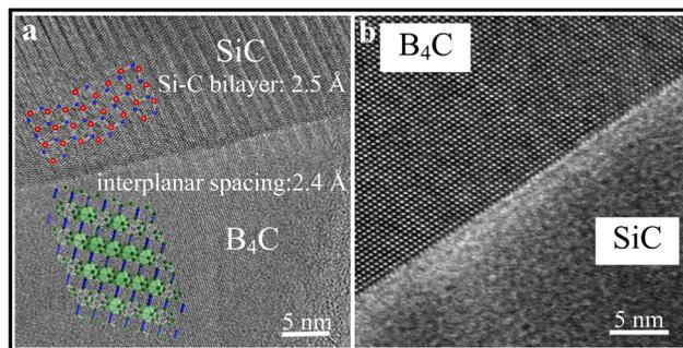
Fig. 8 HRTEM images of B<sub>4</sub>C–SiC ceramics prepared by solid-state sintering revealing the phase boundary characteristics between B<sub>4</sub>C and SiC: (a) B<sub>4</sub>C–40 wt% SiC ceramics with 3 wt% carbon black<sup>136</sup> (reprinted with permission, Copyright 2019, Elsevier) and (b) B<sub>4</sub>C–15 wt% SiC ceramics with 2 wt% carbon black<sup>107</sup> (reproduced with permission, Copyright 2019, Elsevier).
