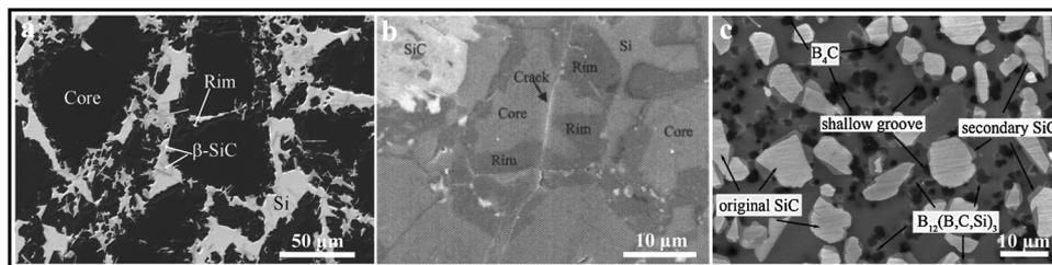
Fig. 9 SEM images of reaction-bonded  $B_4C$ -SiC ceramics exhibiting: (a) core-rim structure of  $B_4C$  particles<sup>137</sup> (reproduced with permission, Copyright 2009, Elsevier), (b) crack propagation path passing through the core-rim structure of  $B_4C$ <sup>138</sup> (reproduced with permission, Copyright 2010, John Wiley and Sons), and (c) core-rim structure of SiC particles<sup>85</sup> (reproduced with permission, Copyright 2016, Elsevier).
