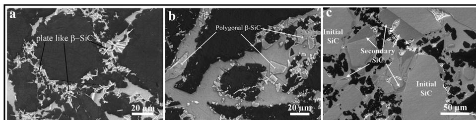
Fig. 10 Morphology of SiC grains in reaction-bonded  $B_4C$ -SiC ceramics produced from the preforms with different compositions: (a)  $B_4C$  without free C addition, (b)  $B_4C$  with 5 wt% free C addition<sup>137</sup> (reproduced with permission, Copyright 2009, Elsevier), and (c) the mixture of  $B_4C$  and SiC without free C addition<sup>143</sup> (reproduced with permission, Copyright 2010, Elsevier).
