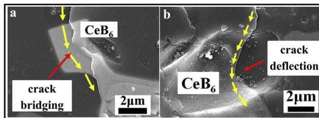
Fig. 16 Crack propagating on the surface of pressureless sintered  $B_4C$ -15 wt% SiC ceramics with the sintering aid of 5 wt%  $CeO_2$ : (a) crack bridging and (b) crack deflection<sup>129</sup> (reproduced with permission, Copyright 2013, Elsevier).
