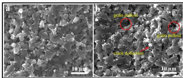
Fig. 14 Fracture surfaces of hot-press sintered  $B_4C$ -20 wt% SiC ceramics at different sintering temperatures: (a) 1800 °C and (b) 1900 °C.<sup>110</sup>
