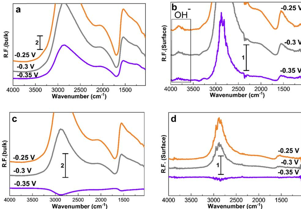
Fig. 7 PM-IRRAS spectra (considering ammonia at  $-0.5$  V as reference) on Pt/C of (a), (b) 1.3 nm size and (c), (d) 2.2 nm particle size during ammonia electro-oxidation in 1 M KOH + 0.5 M  $\text{NH}_4\text{OH}$ . Spectra collected after 30 min at each potential. The left hand side corresponds to the bulk of the electrolyte and the right hand side corresponds to the Pt surface.
