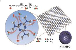
Scalable nitrogen-enriched porous sub-100 nm graphitic carbon nanocapsules for efficient oxygen reduction reaction in different media
