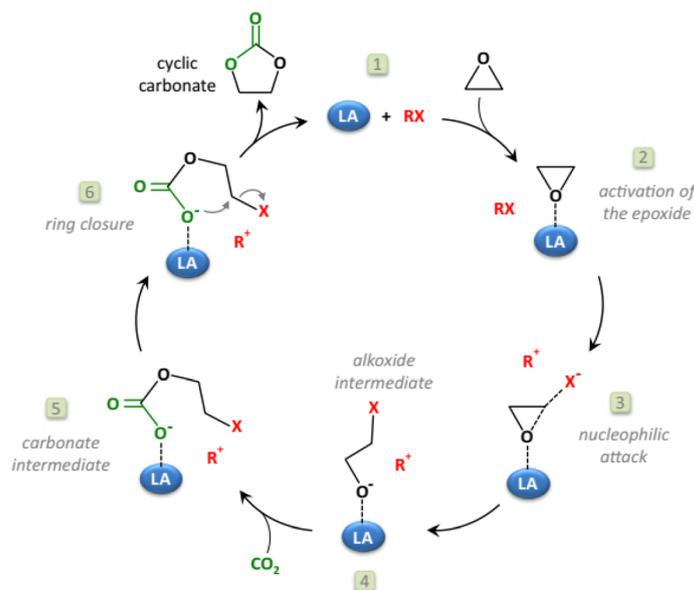
**Scheme 4** The mechanism of coordination of a bifunctional (acid/base) catalyst to an epoxide in the synthesis of alkylene carbonates. Reprinted with permission from "Cyclic carbonates synthesised from CO<sub>2</sub>: applications, challenges and recent research trends" P. P. Pescarmona, *Curr. Opin. Green Sustainable Chem.*, 2021, 29, 100457 (ref. 43), <https://www.sciencedirect.com/science/article/pii/S2452223621000134>.
