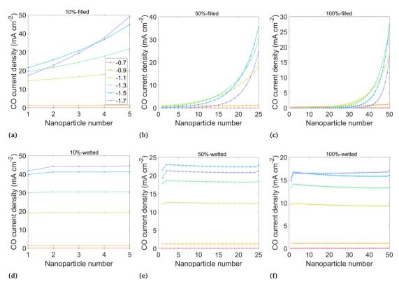
Fig. 5 Average CO current density at the surface of each catalyst nanoparticle at potentials from -0.7 to -1.7 V vs. RHE, for the six wetting cases ((a) -(f) correspond directly to Fig. 3). Nanoparticles are numbered starting at 1 for the left-most (deepest) particle. Current density calculated using catalystelectrolyte surface area.
