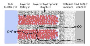
Fig. 8 Cross section of a cathode geometry with alternating layers of gasconducting hydrophobic material and catalyst nanoparticles. The layering geometry would extend the liquid—gas interface, providing a short liquid diffusion length to all catalyst nanoparticles.
