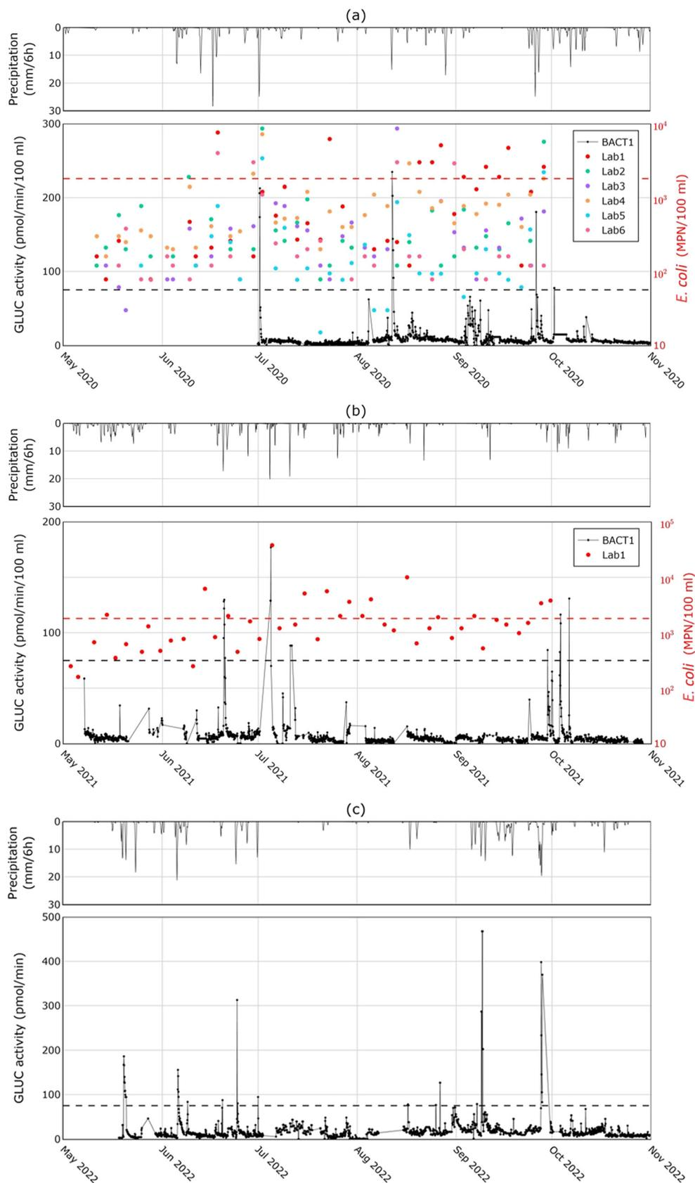
**Fig. 3** a) GLUC activity recorded by the BACTcontrol and measured *E. coli* colonies at all locations in 2020, b) GLUC activity recorded by the BACTcontrol and measured *E. coli* colonies at location LAB 1 in 2021, c) GLUC activity recorded by the BACTcontrol in 2022. The graphs include the 6-hour sum of precipitation *via* radar measurements. The red and black dashed lines show the established hygienic limit values for *E. coli* and GLUC activity, respectively.
