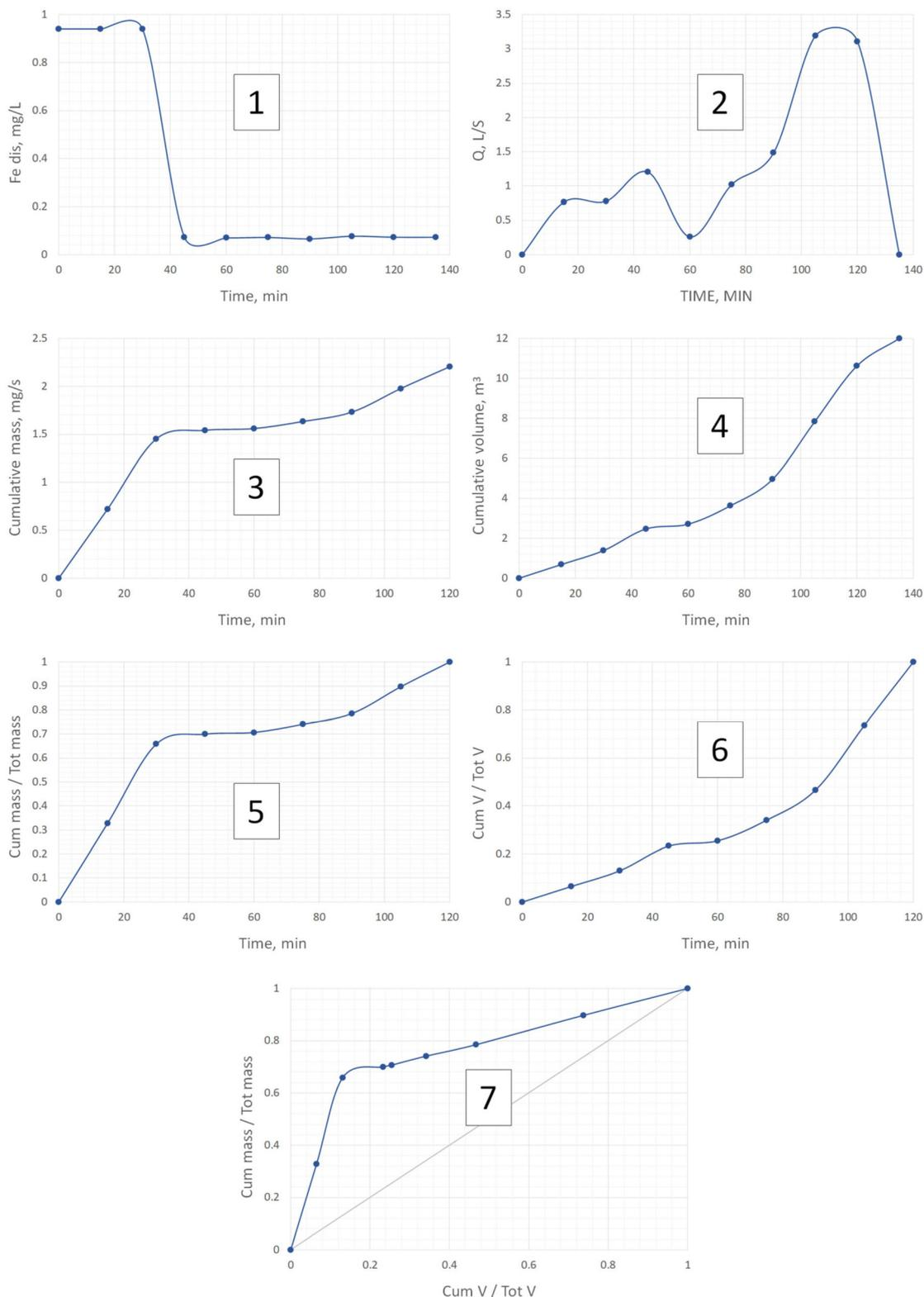
Fig. 4 Example of the drawing of one  $M(V)$  curve for  $Fe_{dis}$  for event 1. The numbers 1-7 indicate the order of drawing each point of the  $M(V)$  curve from both the hydrograph and the pollutograph.
