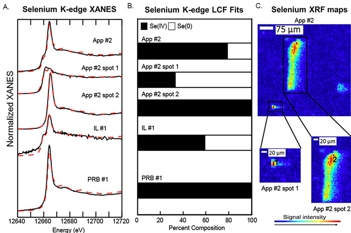
Fig. 5 Selenium speciation in fly ash samples analyzed by bulk and  $\mu$ -XANES. A) Se-XANES spectra data (solid black lines) and model fits (red dotted lines) for bulk and microprobe analysis. B) LCF model results showing percent composition of Se for spectra collected by bulk and  $\mu$ -XANES. C)  $\mu$ -XRF maps of Se showing spots analyzed by  $\mu$ -XANES.
