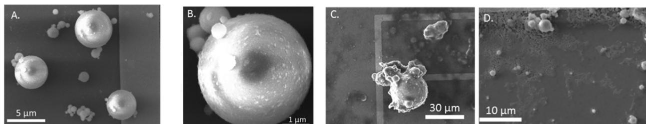
**Fig. 1** SEM images of: A) fly ash sample PRB #1 showing spherical particles of varying sizes; B) a magnified view of PRB #1 showing multiple sized particles clustered together, including  $<1 \mu\text{m}$  particles attached to a  $4 \mu\text{m}$  particle; C) fly ash App #1; D) fly ash App #2.
