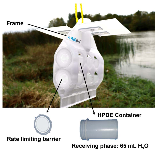
Fig. 1 The components of the equilibrium passive sampler developed in this study.
