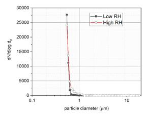
Fig. 11 Size distribution of the PSL aerosol at a nominal diameter of 0.5 μm for the low (≤30%) and high (80%) RH conditions.
