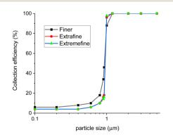
Fig. 3 Collection efficiency curves for a mesh independence study.
