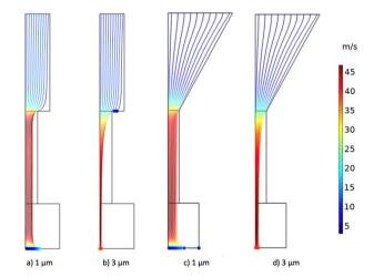
Fig. 6 1  $\mu$ m and 3  $\mu$ m particle trajectories for straight and tapered inlets (the color represents the velocity magnitude).
