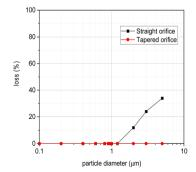
Fig. 5 (a) The collection efficiency curves for the straight and tapered orifice inlets. (b) Calculated particle loss for the two inlet designs.
