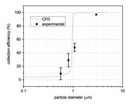
Fig. 10 Particle collection efficiency curve from CFD and experimental data for the microsampler at  $\leq 30\%$  RH.
