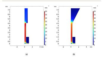
Fig. 4 Gas stream velocity profile for (a) straight orifice and (b) the tapered orifice.
