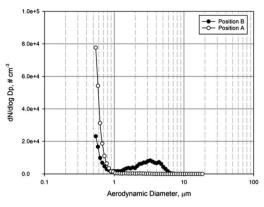
Fig. 12 The size distribution of test aerosol populations in the test chamber at two sampling locations (Note: (A) is the location closer to the chamber exit, while (B) is close to the inlet)
