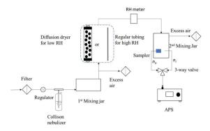
Experimental setup for collection efficiency evaluation
