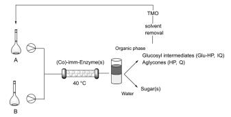
Scheme 2 Flow bioprocessing of HES and RT. Solution A: 10 g L<sup>-1</sup> HES or RT in TMO. Solution B: HEPES buffer, 0.05 M, pH 7.5. Co-immenzyme(s): imm-RN (5 mg  $g_{resin}^{-1}$ ) or HOR (1 mg  $g_{resin}^{-1}$ ) or imm-RN-HOR (5 mg<sub>RN</sub> g<sub>resin</sub><sup>-1</sup>, 1 mg<sub>HOR</sub> g<sub>resin</sub><sup>-1</sup>). T = 40 °C.
