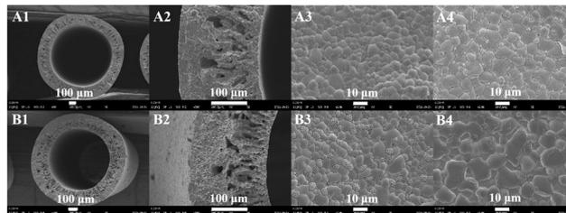
Fig. 5 Microscopic morphology of BCYF<sub>0.10</sub>-YDC/BCYF<sub>0.10</sub>-NiO dual-layer HF membranes sintered at 1600 °C: (A) before reduction, (B) after reduction; (1) cross section, (2) membrane wall, (3) inner surface, (4) outer surface.
