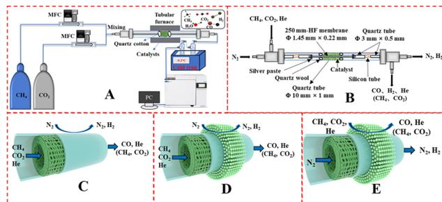
Fig. 3 Schematic illustration of (A) DRM catalytic reactor setup, (B) DRM membrane reactor; gas input method: fiber lumen feeding and shell side sweeping in (C) M1 mode, and (D) M2 mode, (E) shell side feeding and fiber lumen sweeping (M3 mode).
