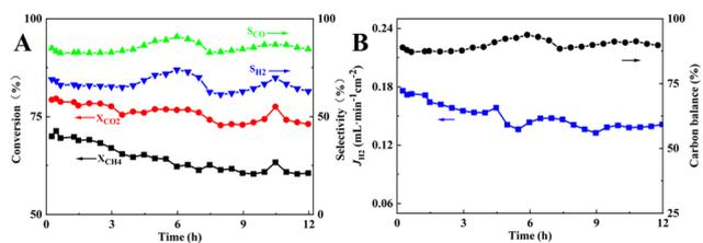
**Fig. 12** Short-term stability of membrane reactor composed of 30 wt% Ni/BCYF<sub>0.10</sub>-YDC catalyst and BCYF<sub>0.10</sub>-YDC/BCYF<sub>0.10</sub>-Ni dual-layer HF membrane in M3 mode at 900 °C: (A) CH<sub>4</sub>, CO<sub>2</sub> conversions and CO, H<sub>2</sub> selectivities; (B) H<sub>2</sub> permeation flux and carbon balance (shell side: 80 mL min<sup>-1</sup> 12.5/12.5/75 vol% CH<sub>4</sub>/CO<sub>2</sub>/He, fiber lumen: 80 mL min<sup>-1</sup> N<sub>2</sub> sweep).
