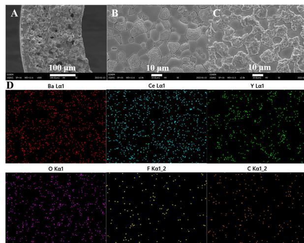
Fig. 8 Microscopic morphology of BCYF<sub>0.10</sub>-YDC/BCYF<sub>0.10</sub>-Ni dual-layer HF membrane after H<sub>2</sub> permeation with CO<sub>2</sub> sweeping: (A) membrane wall, (B) inner surface, (C) outer surface. And (D) corresponding EDS mapping of the outer surface in (C).
