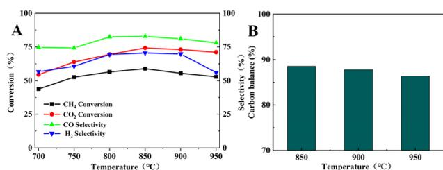
Fig. 9 (A) DRM catalytic performance of BCYF<sub>0.10</sub>-Ni powder, (B) carbon equilibrium (feed gas was 50 mL min<sup>-1</sup> CH<sub>4</sub> and 50 mL min<sup>-1</sup> CO<sub>2</sub>).
