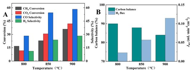
**Fig. 11** (A) CH<sub>4</sub> and CO<sub>2</sub> conversions and CO and H<sub>2</sub> selectivities; (B) carbon balance and H<sub>2</sub> permeation flux of BCYF<sub>0.10</sub>-YDC/BCYF<sub>0.10</sub>-Ni dual-layer HF membranes (fiber lumen: 80 mL min<sup>-1</sup> 12.5/12.5/75 vol% CH<sub>4</sub>/CO<sub>2</sub>/He, shell side: 80 mL min<sup>-1</sup> N<sub>2</sub> sweeping).
