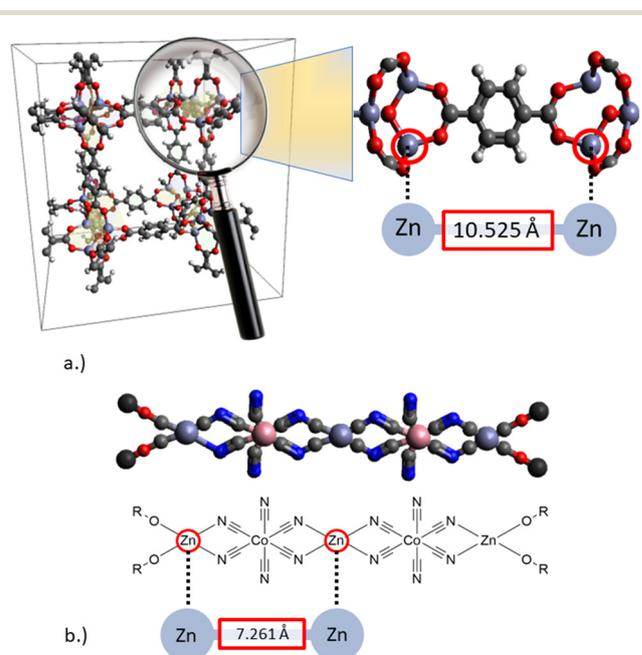
**Fig. 3** Schematic structures of solid bifunctional catalysts for CO<sub>2</sub>/epoxide conversion to cyclic carbonates or linear polycarbonates: a.) metal-organic framework (MOF),<sup>35</sup> b.) double metal cyanide catalysts (DMC).<sup>32</sup>
