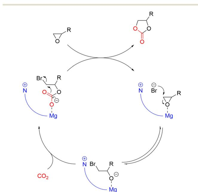
Fig. 1 Mechanism of the formation of cyclic carbonates *via* a bifunctional catalyst system consisting of a Lewis acid and a nucleophile.
