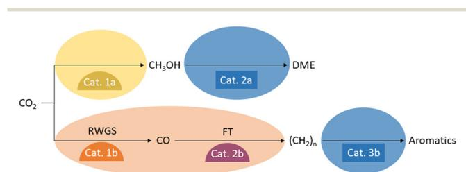
Fig. 4 Hydrocarbon formation by CO<sub>2</sub> hydrogenation via the syngas or methanol route.
