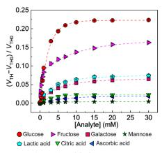
Fig. 3 Response profiles of the GO-OFET-based chemical sensor with 4-MPBA against seven analytes in 0.1 M phosphate buffer with 0.1 M NaCl at pH 7.4. Titration isotherms were obtained by collecting  $V_{TH}$  at each concentration of analytes from 0 to 30 mM. The terms  $V_{\rm TH0}$  and  $V_{\rm TH}$ , respectively, indicate threshold voltages before and after adding the analytes. Three repetitive evaluations were carried out for each analyte.
