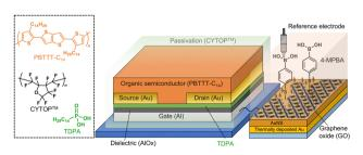
Fig. 1 Schematic illustration of the extended-gate OFET for the monitoring of plasma glucose levels. The extended-gate Au electrode was functionalized with Au nanostructures (AuNSs), graphene oxide (GO), and 4-mercaptophenylboronic acid (4-MPBA).
