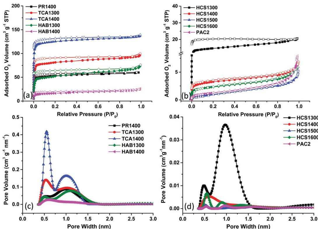
Fig. 1 Hard carbon O<sub>2</sub> adsorption/desorption isotherms (a and b) and the corresponding two-dimensional nonlocal density functional theory (2D-NLDFT) pore size distribution (c and d).
