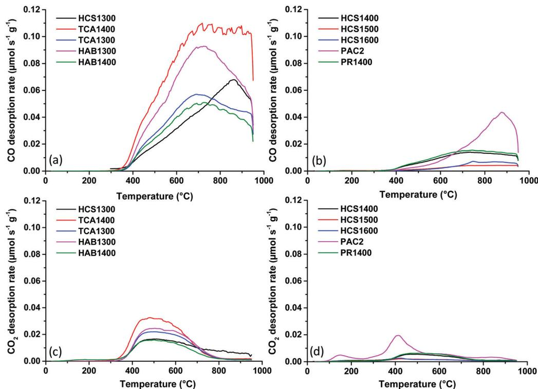
Fig. 2 CO (a and b) and CO<sub>2</sub> (c and d) desorption profiles of hard carbon materials obtained by TPD-MS after the O<sub>2</sub> chemisorption step.
