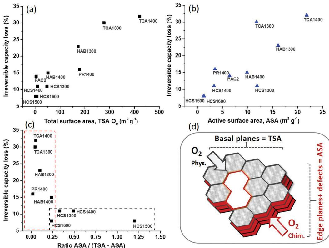
Fig. 3 Relationship between the 1st irreversible capacity loss and (a) total surface area (TSA O<sub>2</sub>), (b) active surface area (ASA), (c) ratio ASA/(TSA O<sub>2</sub>-ASA). (d) Representation of hard carbon structure containing the active surface (edge planes and defects) and the basal planes surface (TSA-ASA).
