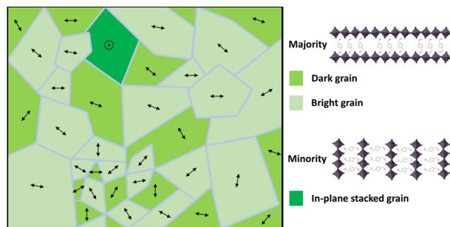
Fig. 6 Schematic of the  $\text{PDMAPbI}_4$  thin film microstructure. Micro-metre sized crystallites predominantly form with layers parallel to the substrate, *i.e.* stacked in out-of-plane direction. These crystallites are rotationally disordered around the stacking direction (indicated by the double-arrows) and can be either bright or dark. A minor sub-population of crystallites forms with their layers perpendicular to the substrate, *i.e.* stacked in in-plane direction.
