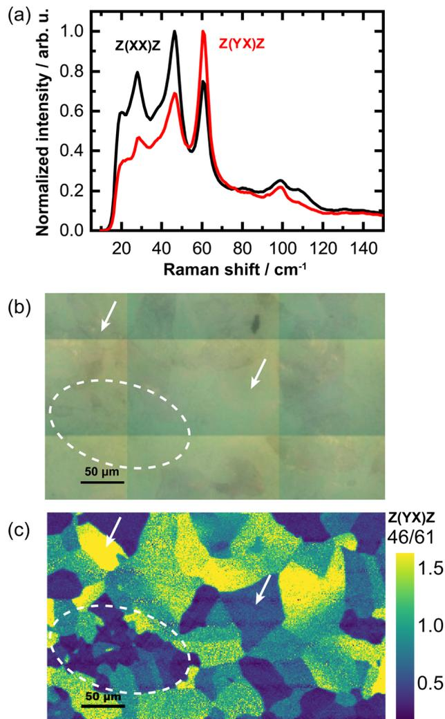
Fig. 4 (a) Average polarised Raman spectra of  $\text{PDMAPbI}_4$  measured in the  $Z(XX)\bar{Z}$  and  $Z(YX)\bar{Z}$  configuration, where the terms inside the brackets indicate the polarisation direction of the incident and detected light, respectively. (b) White light micrograph of the area on which Raman maps were acquired. (c) False colour map showing the ratio of the intensity of the  $46\text{ cm}^{-1}$  peak over the  $61\text{ cm}^{-1}$  peak for the  $Z(YX)\bar{Z}$  polarisation.
