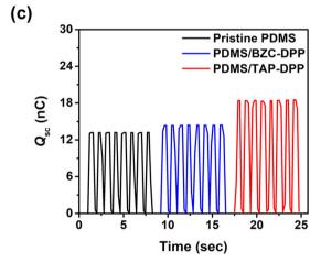
Fig. 5 Output characteristics of resulting TENG: (a)  $V_{\rm oc}$ , (b)  $I_{\rm sc}$ , and (c)  $Q_{\rm sc}$ .
