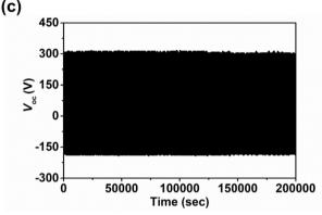
Fig. 7 (a) Output characteristics of resulting TENG as a function of the load resistance. (b) A photograph of 64 LEDs lit up simultaneously by resulting TENG. (c) Evolution of  $V_{\rm oc}$  of resulting TENG as a function of continuous operating cycles under ambient air conditions (25 °C, 50% relative humidity).
