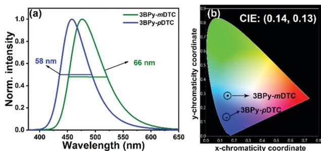
Fig. 4 Blue OLED device based on TADF emitters: (a) electroluminescence (EL) spectra and (b) CIE chromaticity diagram of **3BPpy-pDTC** and **3BPpy-mDTC** depicting the color purity based on the narrow FWHM and CIE coordinates towards pure blue emission.
