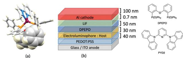
**Fig. 15** (a) Structure of the complex cation in [Cu(POP)(3-Meppzpy)][BF<sub>4</sub>]<sup>+</sup>·0.5CH<sub>2</sub>Cl<sub>2</sub> (CSD refcode VIZKEW) with Ph<sup>·</sup>-arene  $\pi$ -stacking within the POP ligand shown in space-filling representation. (b) Architecture of solution-processed OLEDs with [Cu(POP)(pzpy)][BF<sub>4</sub>]<sup>+</sup> derivatives in the active layer. DPEPO = hole-blocking layer; active layer = 20 wt% Cu-iTMC in either DPEPO or PYD2 as host.
