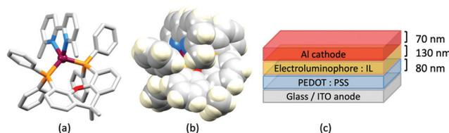
Fig. 7 The structure of the [Cu(xantphos)(6,6'-Me<sub>2</sub>bpy)]<sup>+</sup> cation in the [PF<sub>6</sub>]<sup>-</sup> salt (CSD refcode GABVAJ): (a) with H atoms omitted, and (b) in space-filling representation to show the steric shielding of the Cu(i) centre. (c) Architecture of the LEC devices containing [Cu(xantphos)(N<sup>^</sup>N)][PF<sub>6</sub>] with N<sup>^</sup>N = 6-Mebpy, 6-Etbpy or 6,6'-Me<sub>2</sub>bpy. IL = [EMIM][PF<sub>6</sub>], and Cu-iTMC: IL molar ratio = 4:1.
