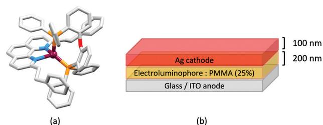
**Fig. 4** (a) The structure of the  $[\text{Cu}(\text{POP})(\mathbf{1})]^+$  cation in  $[\text{Cu}(\text{POP})(\mathbf{1})][\text{BF}_4]$  (CSD refcode GIRJUN) showing the distorted tetrahedral Cu(i) environment and wide-bite angle ( $117.98(3)^\circ$ ) of POP (H atoms are omitted). The phen backbone is rigid ( $\text{N}–\text{Cu}–\text{N} = 80.86(10)^\circ$ ). (b) LEC architecture for a device containing  $[\text{Cu}(\text{POP})(\mathbf{2})][\text{BF}_4]$  as the electrolumiphore.
