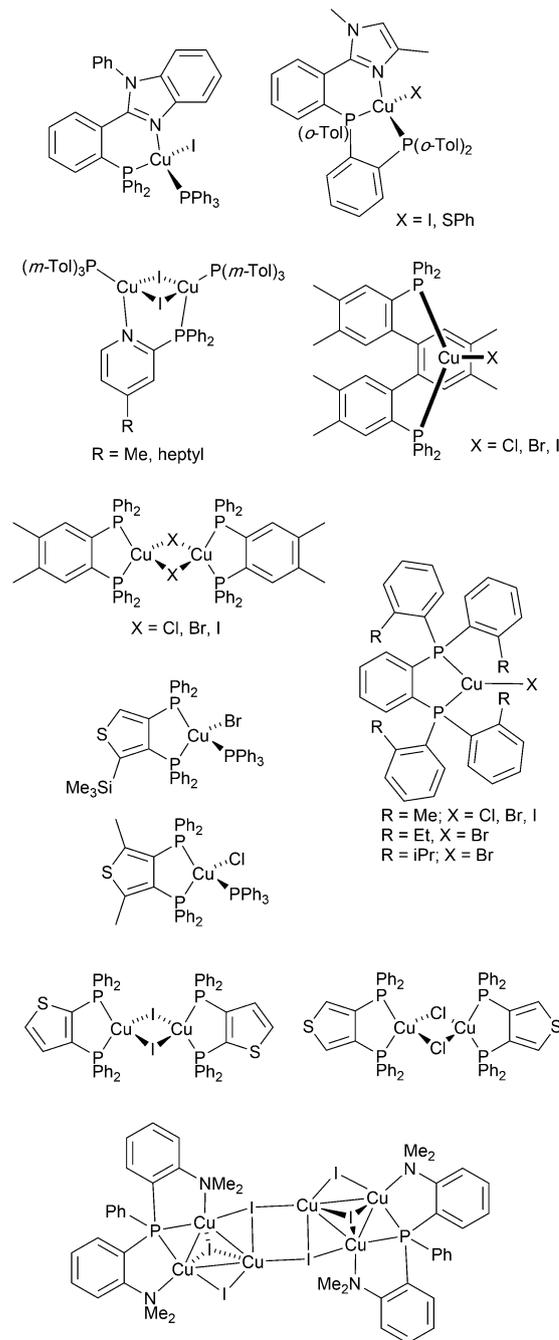
Scheme 3 Structures of selected neutral, TADF copper(i) complexes with Cu–X bonds which have been tested in OLEDs.
