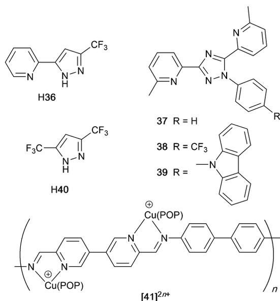
**Scheme 14** Structures of some N<sup>Λ</sup>N or bis(N<sup>Λ</sup>N) ligands in dinuclear Cu(I) complexes, and the structure of metallopolymer **[41]**<sup>2n+</sup>.
