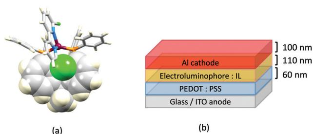
Fig. 10 (a) Structure of the cation in  $[\text{Cu}(\text{xantphos})(6,6'\text{-Cl}_2\text{bpy})][\text{PF}_6]$  (CSD refcode MEWXUK). (b) Architecture of LECs containing the Cu-iTMCs with halogen-substituted bpy ligands.  $\text{IL} = [\text{EMIM}][\text{PF}_6]$  and Cu-iTMC: IL molar ratio = 4 : 1. LECs were driven using a pulsed current.
