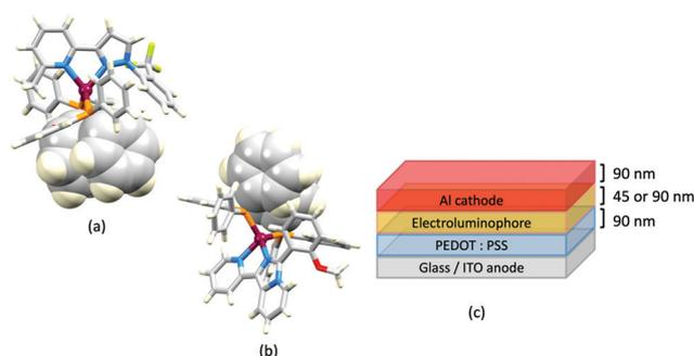
**Fig. 16** Structures of the complex cations in (a) [Cu(POP)(**8**)]<sup>+</sup>[BF<sub>4</sub>]<sup>−</sup>·EtOH (CSD refcode JUFNOP) and (b) [Cu(POP)(**11**)]<sup>+</sup>[PF<sub>6</sub>]<sup>−</sup> showing Ph<sup>·</sup>-arene  $\pi$ -stacking in the POP ligand (space-filling representation). (c) LEC architecture for testing with [Cu(POP)(**11**)]<sup>+</sup>[PF<sub>6</sub>]<sup>−</sup> in the active layer; LECs were driven with a pulsed current.
