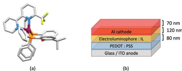
Fig. 11 (a) Structure of the  $[\text{Cu}(\text{xantphos})(6\text{-CF}_3\text{bpy})]^+$  cation in the  $[\text{PF}_6]^-$  salt (CSD refcode VICQUW); the  $6\text{-CF}_3$  bpy ligand is disordered over two sites and only the major occupancy site is shown. H atoms are omitted. (b) Architecture of LECs containing the Cu-iTMCs with  $\text{CF}_3$ -functionalized bpy ligands.  $\text{IL} = [\text{EMIM}][\text{PF}_6]$  and Cu-iTMC: IL molar ratio = 4 : 1. LECs were driven using a pulsed current.
