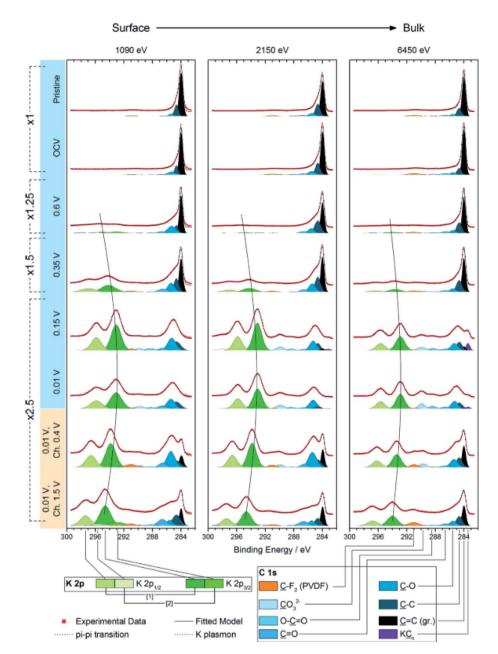
Fig. 16 K 2p – C 1s XPS spectra measured using SOXPES/HAXPES for graphite electrodes at various states of charge from carbonate-based electrolytes. Reprinted with permission from ref. 149. Copyright 2015 American Chemical Society.
