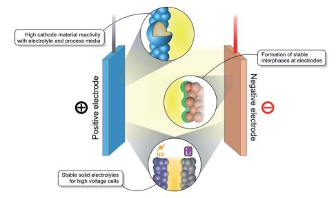
Fig. 1 Schematic diagram demonstrating the interfacial challenges generally found in rechargeable batteries. These mostly include cathode reactivity with electrolyte and process media, formation of stable interphases, and creation of stable interfaces between solid electrolytes and high-voltage electrodes
