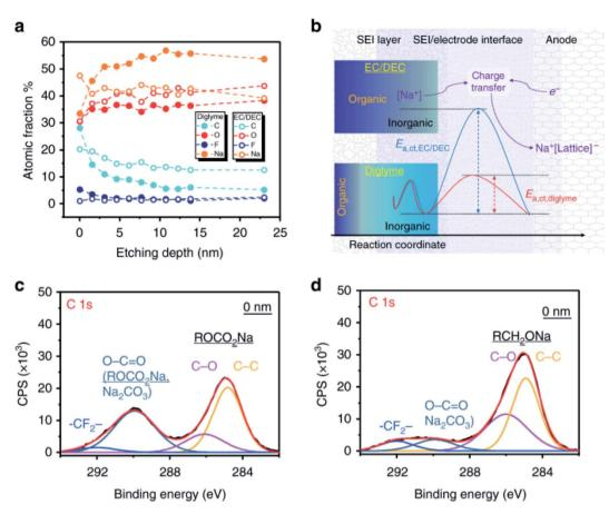
Fig. 14 (a) Quantitative analysis of XPS data from sputtering depth profiling of the SEI formed from ether and carbonate electrolytes. (b) Schematic diagrams for the SEI composition. (c) C 1s spectrum for the electrode with carbonate-SEI before sputter-etching. (d) C 1s spectrum for the electrode with ether-SEI before sputter-etching. Reproduced under CC-BY licence from ref. 144.
