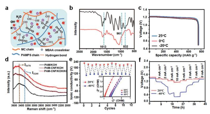
Fig. 10 (a) Schematic diagram of the PAMPS-K/MC hydrogels. (b) FT-IR spectra of the freeze-dried PAMPS/MC hydrogels (red) and the mixture of AMPS/MC (black). (c) Specific capacity of the ZABs at different temperatures. Reproduced with permission from ref. 97. Copyright 2021, American Chemical Society. (d) Raman spectra. (e) Ionic conductivity at 20 and -40 °C. (f) Rate performance. Reproduced with permission from ref. 101. Copyright 2021, Elsevier.
