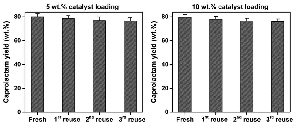
Fig. 9 Reusability of the spent SSWC-CO<sub>2</sub> catalyst with different catalyst loadings for the thermocatalytic conversion of FNW at 500 °C under a CO<sub>2</sub> environment.
