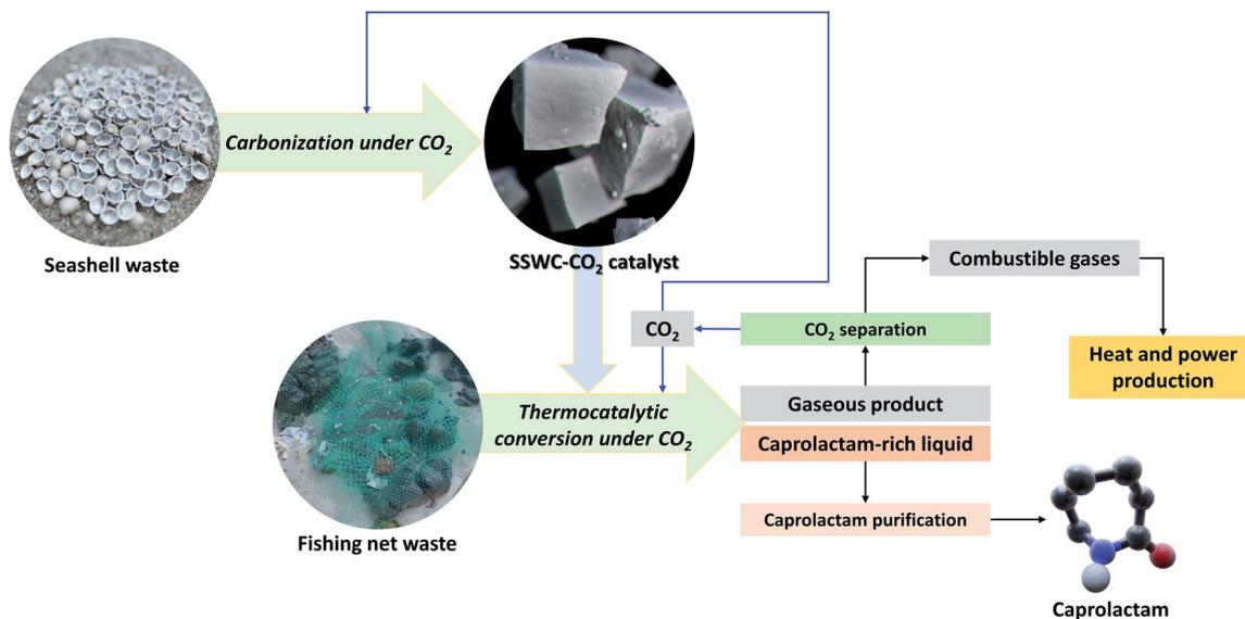
Fig. 10 Concept underpinning the thermocatalytic upcycling of marine waste (FNW and seashell waste) to monomer (caprolactam) under a CO<sub>2</sub> environment with the recycling of by-products.
