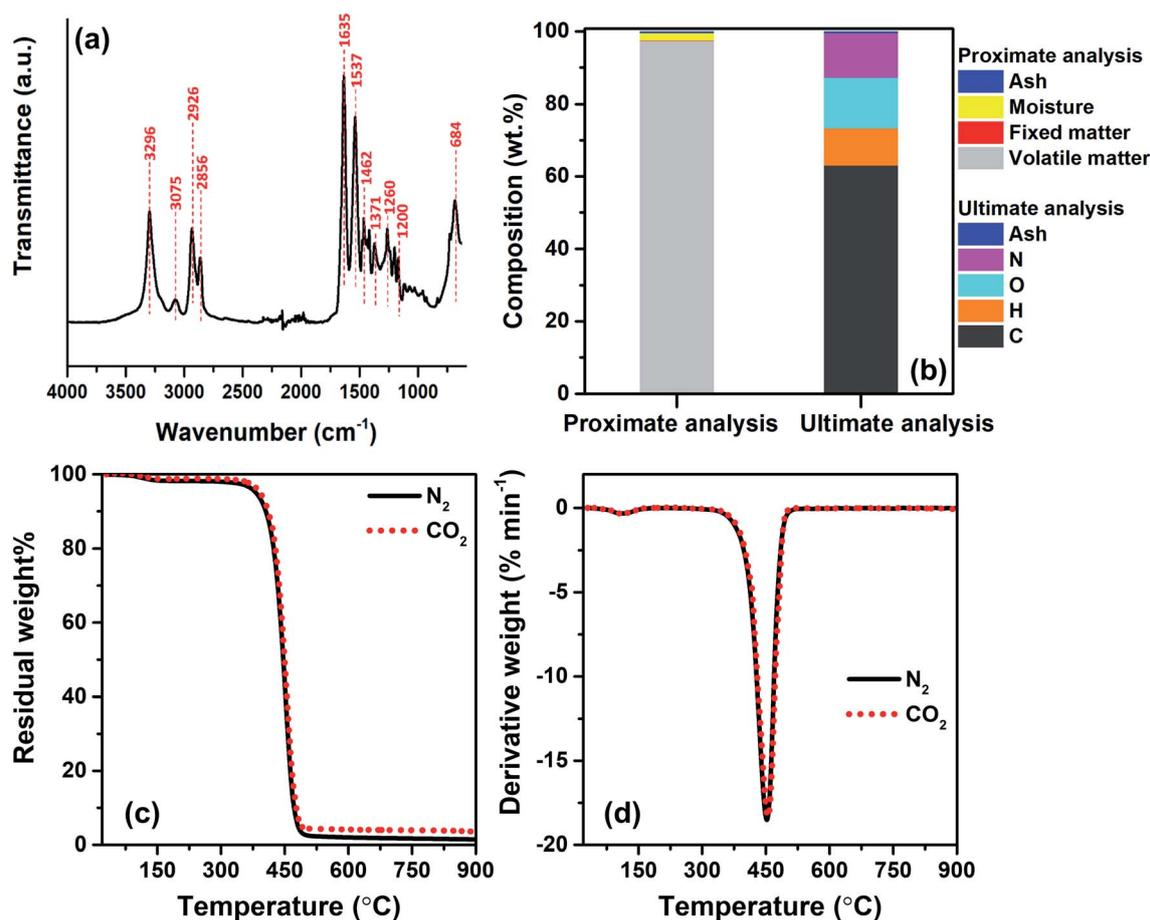
Fig. 2 (a) FTIR spectrum of FNW; (b) proximate and ultimate analyses results of FNW; (c) residual mass change in terms of temperature for the TGA of FNW under  $N_2$  and  $CO_2$  environments; and (d) derivative weight variation in terms of temperature for the TGA of FNW under  $N_2$  and  $CO_2$  environments.
