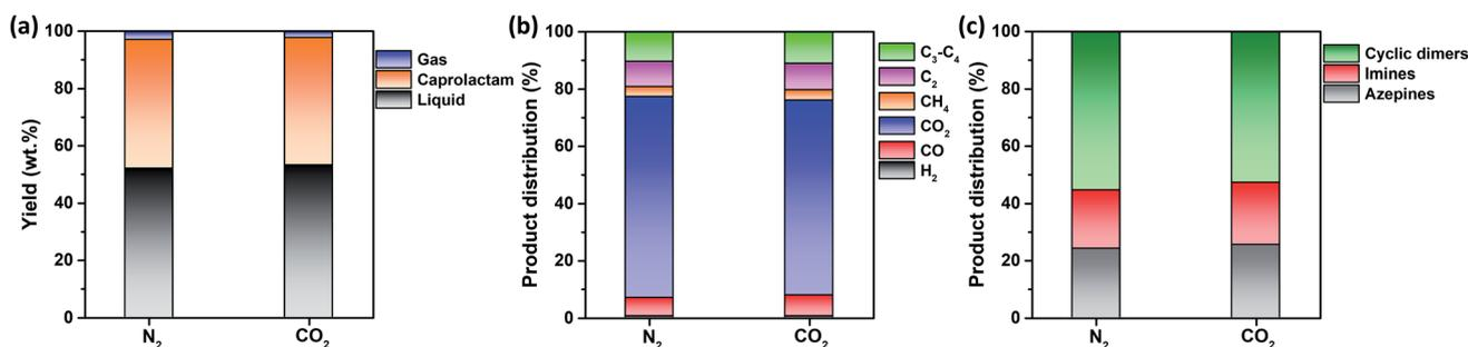
Fig. 3 (a) Yields of gaseous and liquid products, and caprolactam produced from the non-catalytic thermal conversion of FNW at 500 °C under  $N_2$  and  $CO_2$  environments; (b) distribution of gaseous products; (c) distribution of liquid products.
