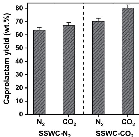
Fig. 8 Caprolactam yield from the thermocatalytic conversion of FNW at 500 °C under N<sub>2</sub> and CO<sub>2</sub> environments using SSWC-N<sub>2</sub> and SSWC-CO<sub>2</sub> in an *in situ* catalyst configuration.
