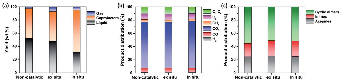
Fig. 6 (a) Yields of gaseous and liquid products, and caprolactam produced from the thermocatalytic conversion of FNW at 500 °C under an  $\text{N}_2$  environment using SSWC- $\text{N}_2$  in different catalyst configurations; (b) distribution of gaseous products; (c) distribution of liquid products.
