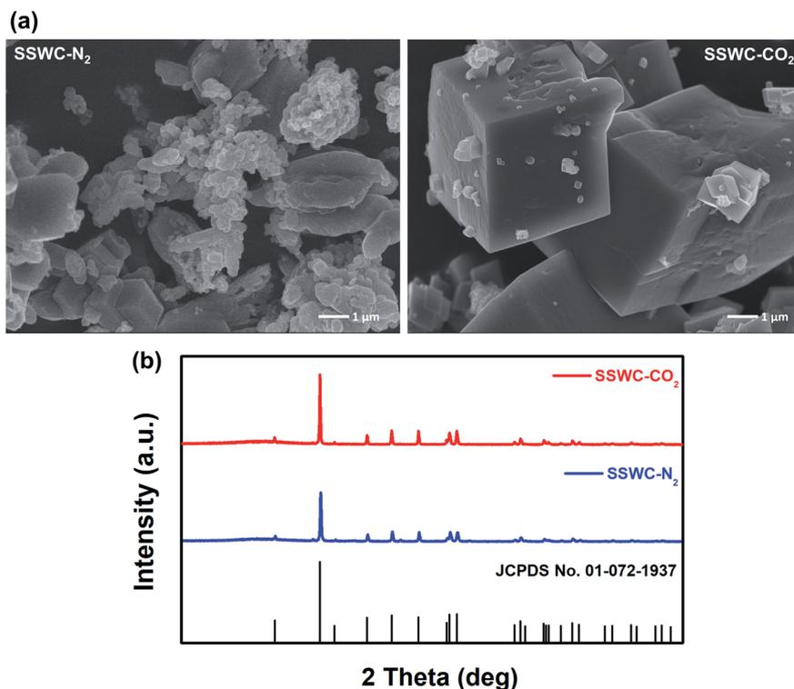
Fig. 5 (a) Scanning electron microscopy (SEM) images of SSWC-N<sub>2</sub> and SSWC-CO<sub>2</sub> (SEM images with a magnification of 5 μm are given in Fig. S7†); (b) XRD patterns of SSWC-N<sub>2</sub> and SSWC-CO<sub>2</sub>.
