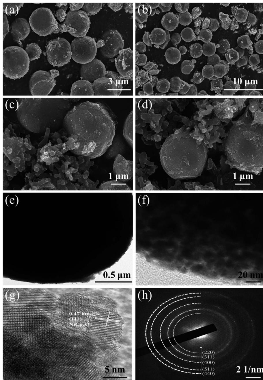
Fig. 5 SEM images of (a and b)  $\text{NiCo}_2\text{O}_4$  nanospheres at different scales. (c and d) The PANI/ $\text{NiCo}_2\text{O}_4$  composite. TEM images of (e and f)  $\text{NiCo}_2\text{O}_4$  nanospheres at different magnifications. (g) HRTEM images of  $\text{NiCo}_2\text{O}_4$  nanospheres. (h) The corresponding SAED pattern of  $\text{NiCo}_2\text{O}_4$  nanospheres.
