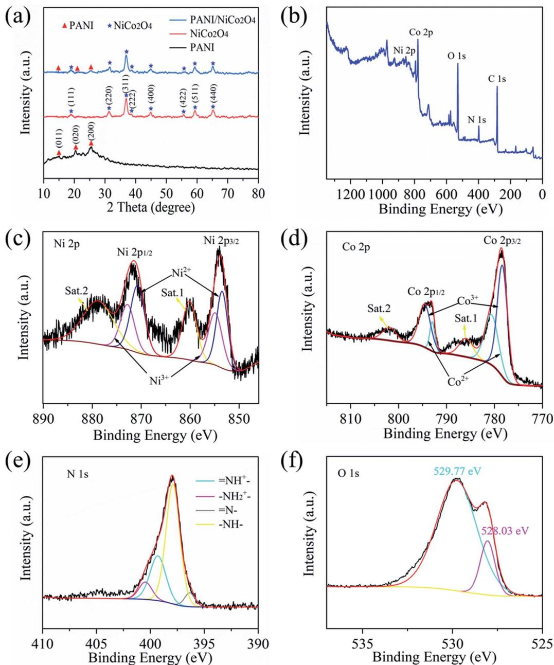
Fig. 6 (a) XRD pattern of pure PANI, pure  $\text{NiCo}_2\text{O}_4$  and the PANI/ $\text{NiCo}_2\text{O}_4$  composite. XPS spectra of the PANI/ $\text{NiCo}_2\text{O}_4$  composite: the (b) survey spectrum, (c) Ni 2p spectrum, (d) Co 2p spectrum, (e) N 1s spectrum and (f) O 1s spectrum.
