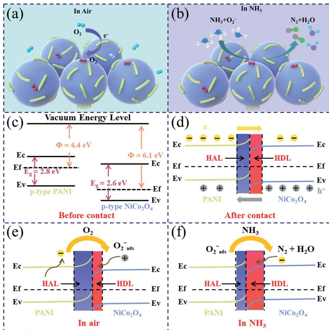
Fig. 8 (a and b) Gas adsorption and desorption processes on the surface of  $\text{NiCo}_2\text{O}_4$  nanospheres in air and  $\text{NH}_3$ , respectively. (c and d) The energy band diagram of PANI and  $\text{NiCo}_2\text{O}_4$  before and after contact, respectively. (e and f) The energy band structure of the PANI/ $\text{NiCo}_2\text{O}_4$  heterojunction exposed to air and  $\text{NH}_3$ , respectively.
