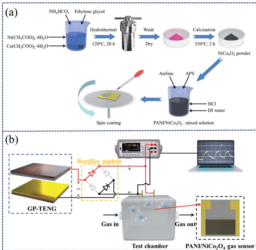
Fig. 2 (a) The diagram of preparation process of the NH<sub>3</sub> gas sensor based on the PANI/NiCo<sub>2</sub>O<sub>4</sub> composite. (b) The experimental test platform of the self-powered GPAS based on the PANI/NiCo<sub>2</sub>O<sub>4</sub> composite.
