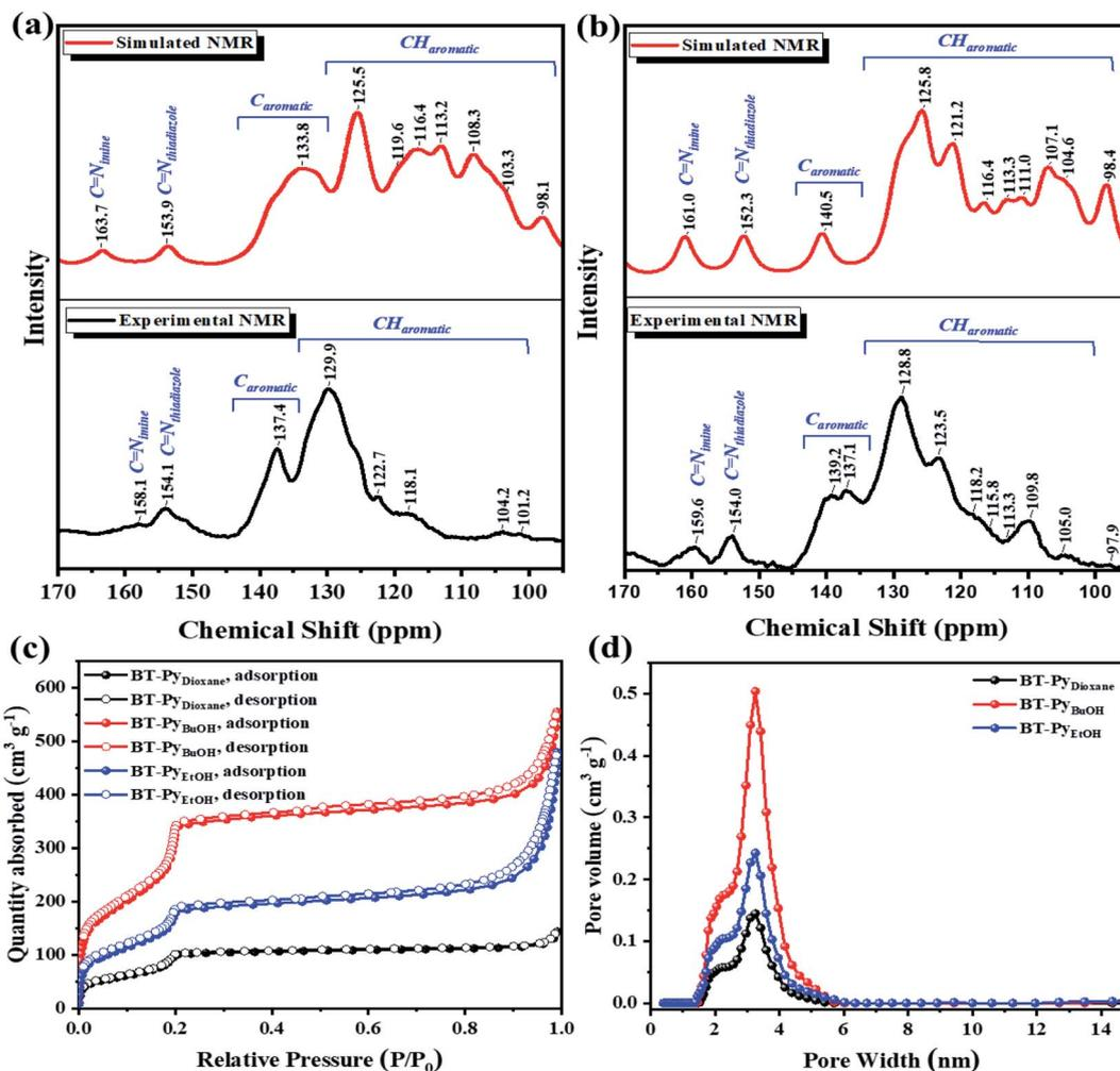
Fig. 2 Simulated and experimental <sup>13</sup>C-NMR spectra of the (a) BT-Py<sub>Solvent</sub> COFs and (b) BT-Cz<sub>Solvent</sub> COFs. (c) N<sub>2</sub> adsorption (solid symbols) and desorption (open symbols) isotherms of the BT-Py<sub>Solvent</sub> COFs at 77 K. (d) The pore-size distribution of the BT-Py<sub>Solvent</sub> COFs.
