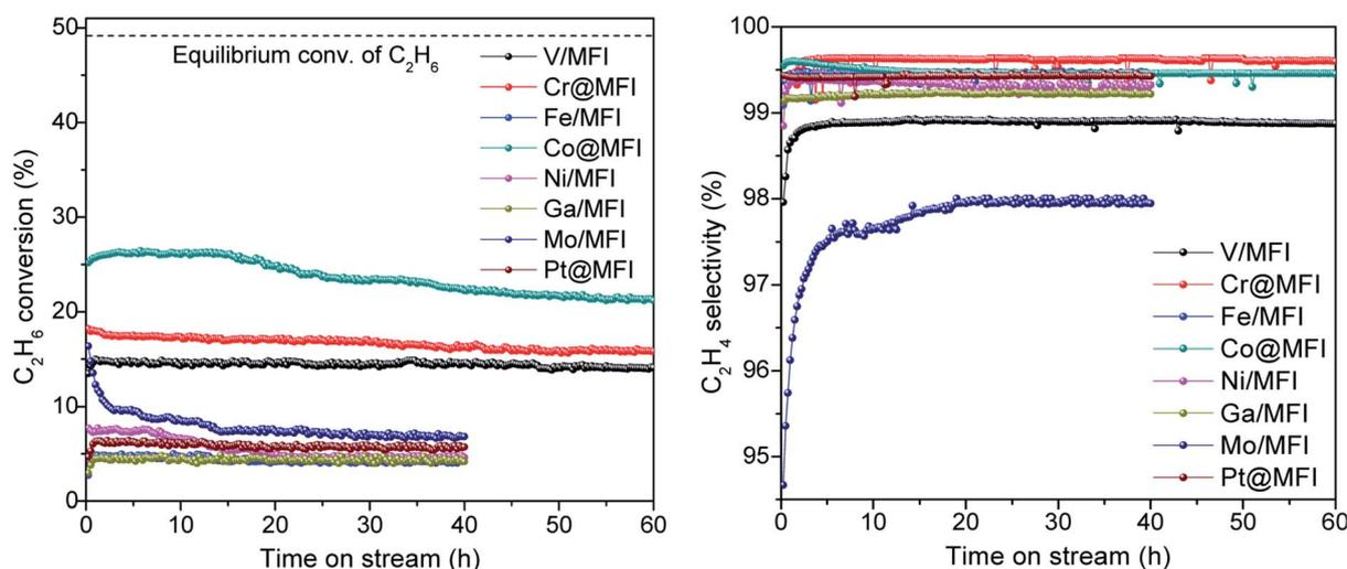
Fig. 1 EDH activities of different metal catalysts. Reaction conditions: 100 mg catalyst, pretreatment by 10%  $\text{H}_2/\text{N}_2$  for 30 min, 20%  $\text{C}_2\text{H}_6/\text{N}_2$ , 10  $\text{mL min}^{-1}$ , 1 bar, 650 °C.
