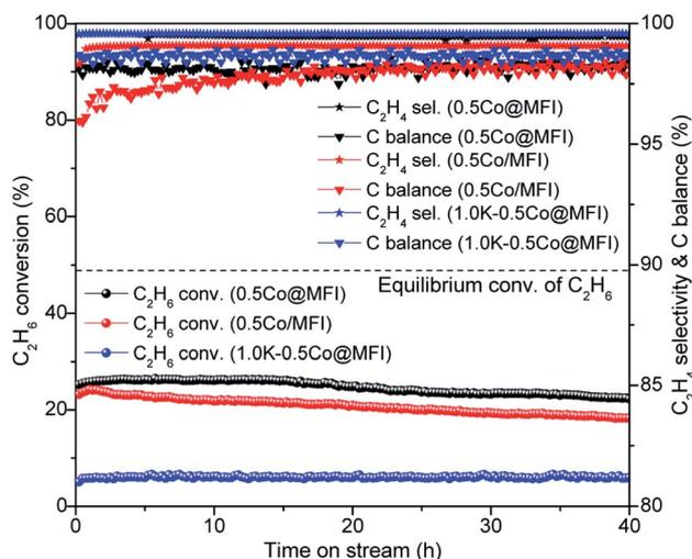
Fig. 6 EDH performances of 0.5Co@MFI, 0.5Co/MFI, and 1.0K-0.5Co@MFI at 1 bar pressure. Reaction conditions: 100 mg catalyst, pretreatment by 10%  $\text{H}_2/\text{N}_2$  for 30 min, 20%  $\text{C}_2\text{H}_6/\text{N}_2$ , 10  $\text{mL min}^{-1}$ , 650 °C.
