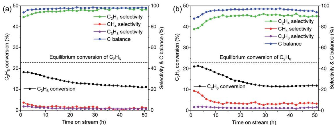
Fig. 8 Catalytic performances of (a) 0.5Co@MFI and (b) 1.3Co@MFI catalysts at 7.5 bar pressure. Reaction conditions: 50 mg catalyst, pretreatment by 10% H<sub>2</sub>/N<sub>2</sub> for 30 min, 20% C<sub>2</sub>H<sub>6</sub>/N<sub>2</sub>, 5 mL min<sup>-1</sup>, 650 °C.
