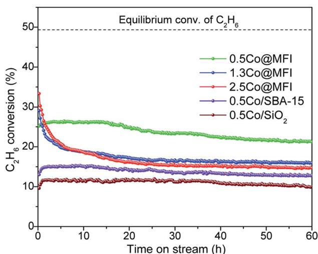
Fig. 5 Effect of Co loading and catalyst support on the EDH activities of different Co catalysts. Reaction conditions: 100 mg catalyst, pretreatment by 10%  $\text{H}_2/\text{N}_2$  for 30 min, 20%  $\text{C}_2\text{H}_6/\text{N}_2$ , 10  $\text{mL min}^{-1}$ , 1 bar, 650 °C.
