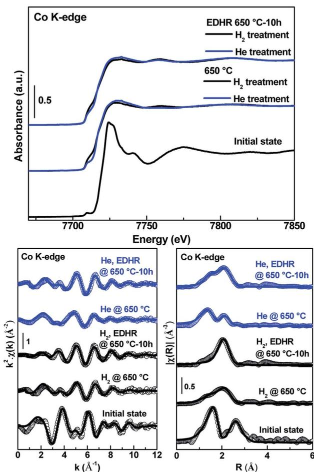
Fig. 9 Evolution of Co K-edge XANES spectra (top) of 0.5Co@MFI at the initial state, after pretreatment, and after EDHR.  $k^2$  weighed EXAFS spectra (bottom left) and FTs (bottom right) of 0.5Co@MFI at the initial state, after H<sub>2</sub> pretreatment, and after EDHR.
