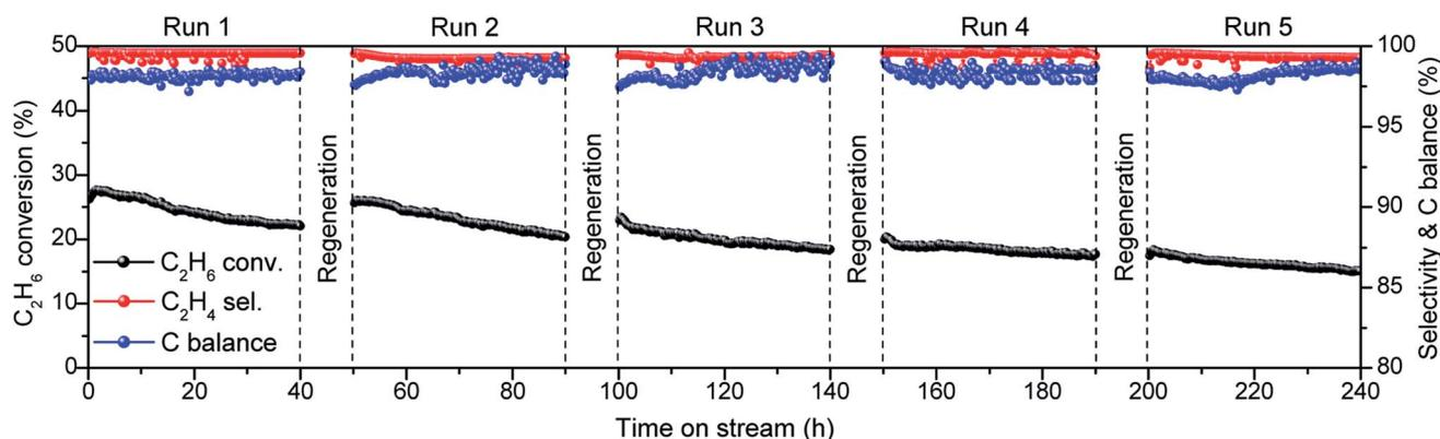
Fig. 7 Recycling experiment with 0.5Co@MFI catalyst. Reaction conditions: 100 mg catalyst, pretreatment by 10% H<sub>2</sub>/N<sub>2</sub> for 30 min, 20% C<sub>2</sub>H<sub>6</sub>/N<sub>2</sub>, 10 mL min<sup>-1</sup>, 1 bar, 650 °C.
