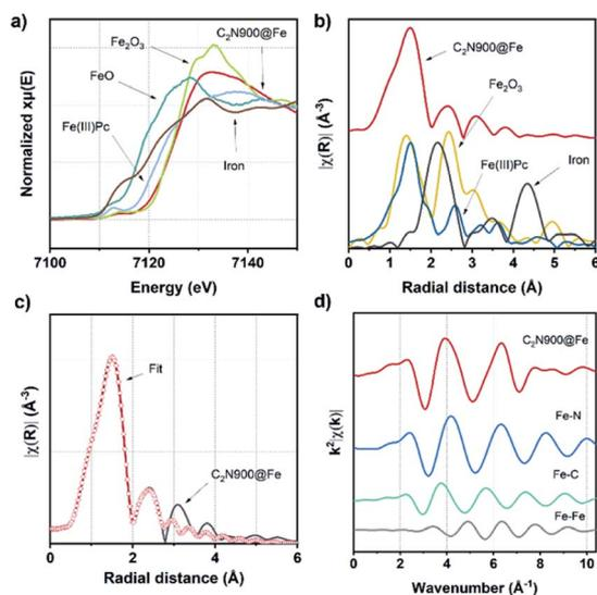
Fig. 3 XANES spectra (before electrochemical measurements) of  $C_2N900@Fe$ ,  $Fe(III)Pc$ ,  $Fe_2O_3$ ,  $FeO$  and  $Fe$  foil (a). FT of  $Fe$  K-edge EXAFS spectra of  $C_2N900@Fe$ ,  $FePc$ ,  $Fe_2O_3$ ,  $FeO$  and  $Fe$  foil (b). The magnitude of EXAFS FT  $k_2$ -weight  $Fe$  K-edge spectra and fitting curve of  $C_2N900@Fe$  (c) and  $q$  space of  $C_2N900@Fe$  and  $Fe-N$ ,  $Fe-C$ , and  $Fe-Fe$  paths (d).
