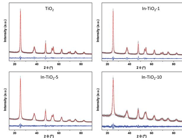
Fig. 1 Pawley refinement of X-ray diffractograms of In-doped and bare TiO<sub>2</sub> samples. Circles: experimental data; red line: fitting; grey line: background; blue line: experiential-simulation subtraction.
