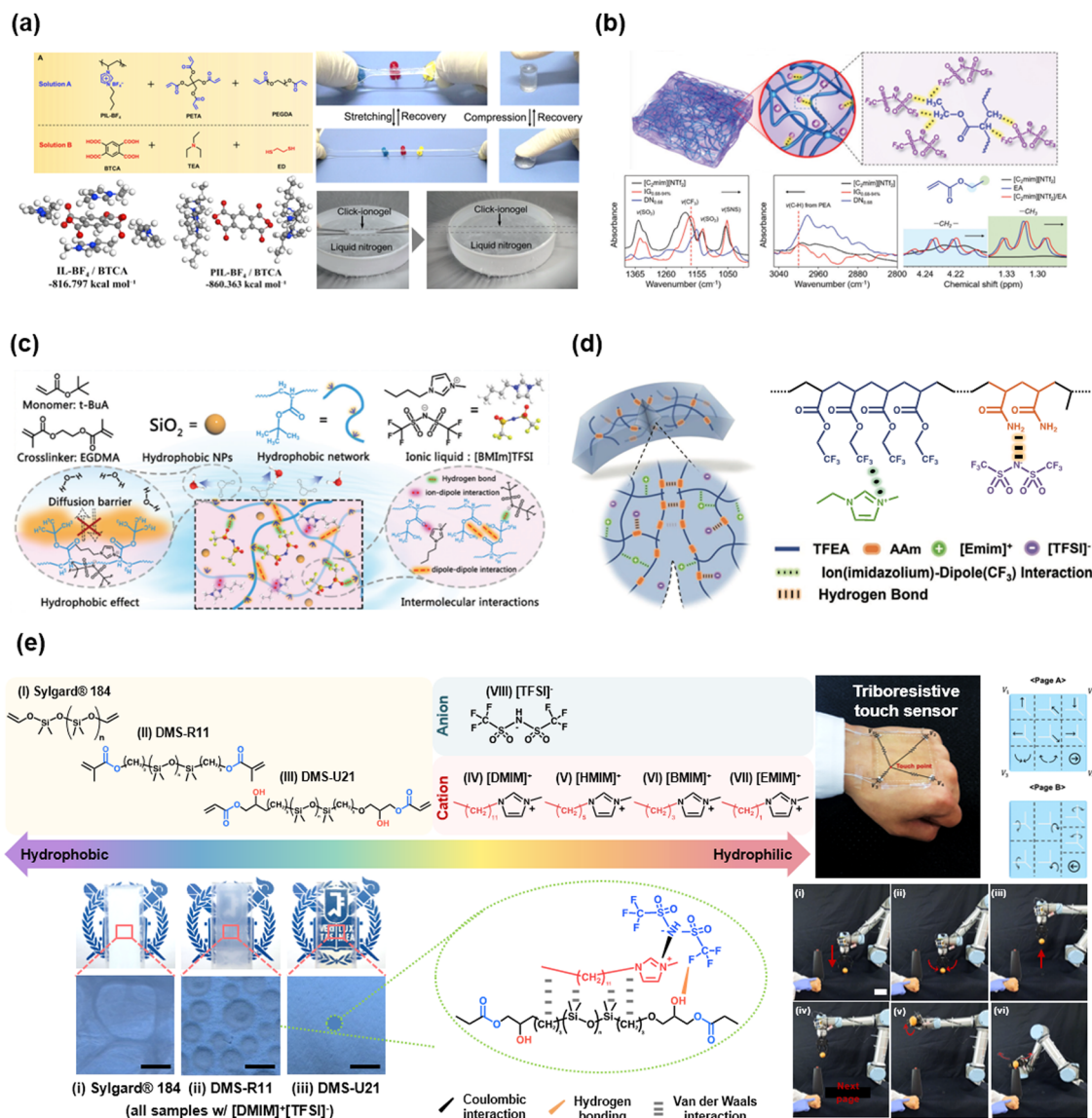
Fig. 9 Representative acrylate or oligomer based IL-SICs. (a) Thiol-ene cross-linked double network click ionogels for stable iononics. Reproduced with permission from ref. 101. Copyright 2019, AAAS. (b) Ethyl acrylate (EA) based double network ionogels, stabilized by hydrogen bonding between the alkyl group and ILs. Reproduced with permission from ref. 92. Copyright 2020, The Royal Society of Chemistry. (c) A fully hydrophobic IL-SICs for underwater communications. Reproduced with permission from ref. 99. Copyright 2021, The Royal Society of Chemistry. (d) Self-healable IL-SICs through hydrogen bonding and ion-dipole interaction. Reproduced with permission from ref. 100. Copyright 2021, Wiley-VCH. (e) Ionic PDMS, which is based on hydrophilic PDMS and hydrophobic IL through hydrogen bonding and van der Waals interaction for triboresistive touch sensors. Reproduced with permission from ref. 91. Copyright 2022, Wiley-VCH.
