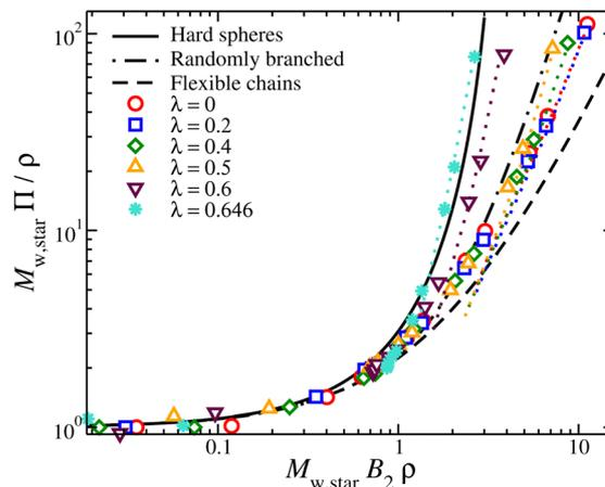
Fig. 8 Compressibility factor,  $M_{w, \text{star}} \Pi / \rho$ , for compact nanogel particles (dotted lines) and star polymer solutions (symbols), as a function of  $B_2 M_w \rho$  for different values of solvent quality parameter,  $\lambda$ . The cases of hard spheres based on the Carnahan–Starling,<sup>71</sup> flexible chains,<sup>72</sup> and randomly branched structures<sup>56</sup> are also presented.
