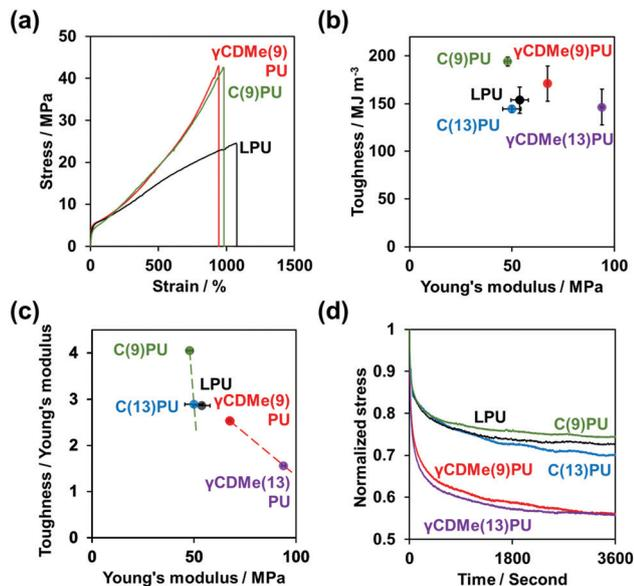
Fig. 3 (a) Stress–strain curves, (b) plots of toughness versus Young's modulus, (c) plots of toughness divided by Young's modulus and Young's modulus, and (d) relaxation time curves of LPU,  $\gamma$ CDMe(*x*)PU, and C(*x*)PU. The  $\gamma$ CDMe(*x*)PU showed higher fracture stress, Young's modulus, and shorter relaxation times than the LPU and C(*x*)PU.
