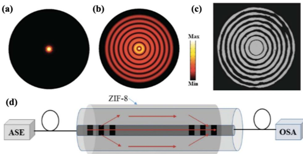
Fig. 13 (a) Optical power distribution of the fundamental mode (LP<sub>01</sub>, core mode) and (b) higher-order mode (LP<sub>08</sub>, cladding mode); (c) near-field image of the LP<sub>08</sub> mode pattern obtained with an infrared camera; (d) schematic diagram of the proposed fibre interferometer with cascaded LPGs. ASE: amplified spontaneous emission light source; OSA: optical spectrum analyzer.<sup>119</sup>
