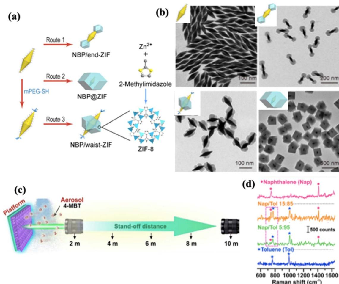
Fig. 15 (a) Schematics of the routes for selective deposition of ZIF-8 on the Au NBPs. (b) TEM images of the Au NBPs, NBP/end-ZIF, NBP/waist-ZIF, and NBP@ZIF nanostructures, respectively.<sup>194</sup> (c) Illustration of the setup for stand-off SERS sensing. (d) Stand-off multiplex spectra obtained under outdoor conditions with natural light, for two different mixtures of naphthalene and toluene, with reference to individual naphthalene and toluene SERS spectra.
