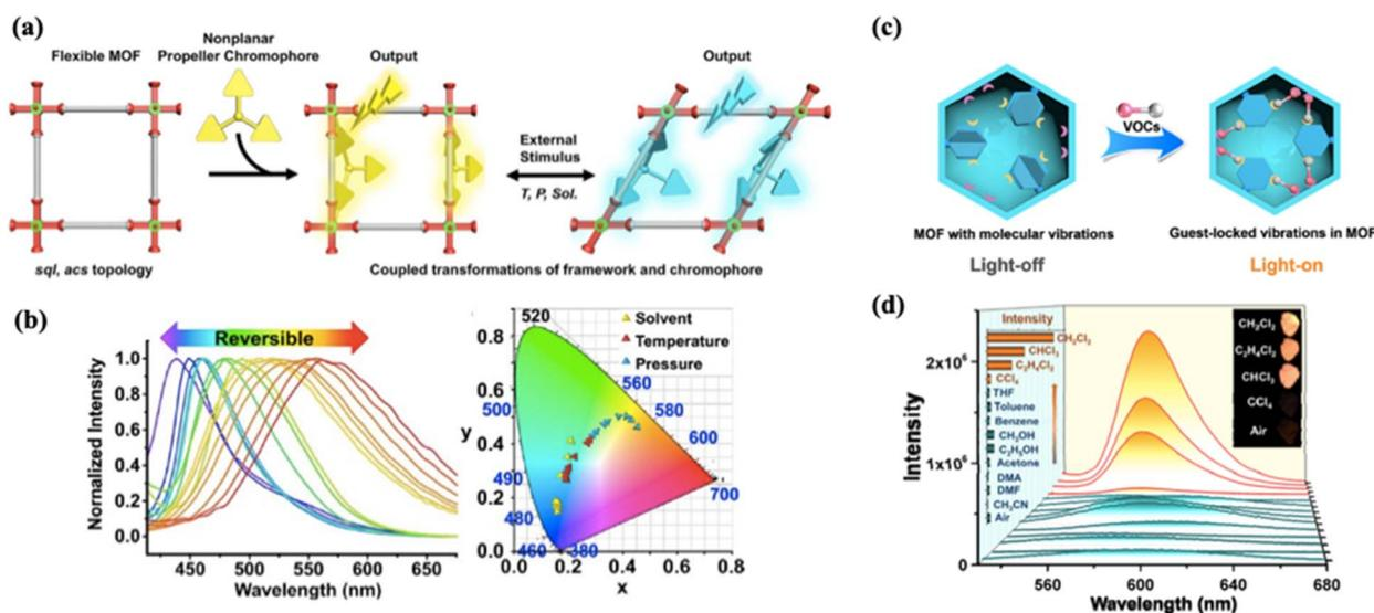
Fig. 7 (a) Illustration of the organic chromophore 3-TPPA grafted in the dynamic coordination space of a flexible MOF. (b) Wide-range emission colour tuning of a 3-TPPA grafted MOF-105 material.<sup>107</sup> (c) Illustration of the guest-induced luminescence enhancement mechanism in the presence of VOCs. (d) Emission spectra of  $[\text{Cu}_4\text{I}_4(\text{Py}_3\text{P})_2]_n$  after incubation for 30 min in various solvent vapours.<sup>108</sup>
