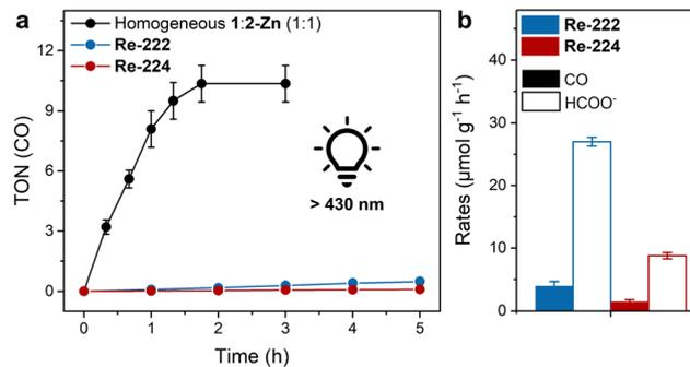
Fig. 3 Photocatalytic CO<sub>2</sub> reduction performance. (a) TON(CO) vs. time plot for MOF samples, including the homogeneous reference (black trace). (b) Product evolution rates averaged over the first two irradiation hours. Standard conditions: MOF sample (1.5 mg) suspended in MeCN (4 mL) and deionised H<sub>2</sub>O (0.12 mL) with BIH (225 mg), room temperature, continuous  $>430$  nm irradiation.
