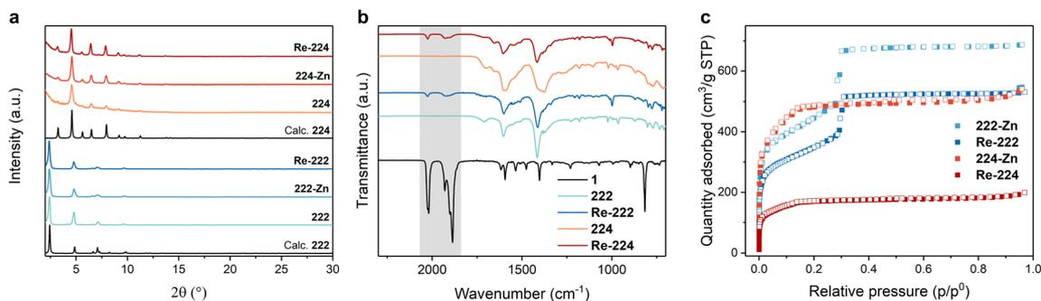
Fig. 2 Material characterisation for pristine and loaded PCN-222 and PCN-224 assemblies. (a) Measured PXRD data. (b) ATR-IR spectra including the reference for pure catalyst **1** (black trace) and with the characteristic region for Re(CO)<sub>3</sub> bands highlighted in grey. Full spectra in ESI.† (c) N<sub>2</sub> sorption isotherms at 77 K.
