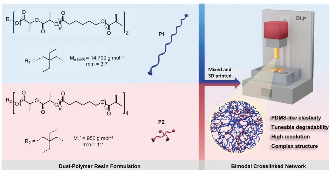
**Scheme 1** Schematic of the strategy for 3D printing of biodegradable elastomers using P1/P2 dual-polymer resins. Dual-polymer resins were designed by combining two distinct poly(DLLA-co-CL) MAs in various weight ratios.  $M_n^*$  represents the highest peak of the MALDI-TOF spectrum of P2.
