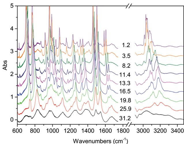
**Fig. 1** Representative spectra showing the evolution of the IR absorption spectrum of the TS crystal with increasing pressure at ambient temperature. The pressure values reported are expressed in GPa.
