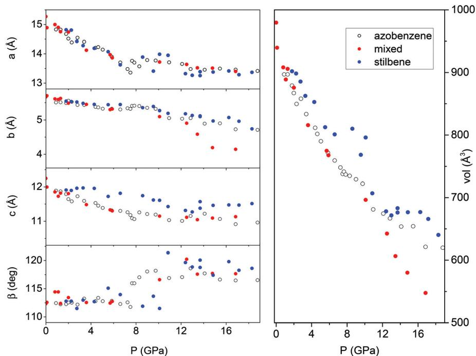
**Fig. 8** Pressure evolution of the lattice parameters as derived by Le Bail refinement of the XRD integrated patterns of TA, TS and TS–TA mixed crystals all compressed without the pressure transmitting medium. The data for TA crystals are from ref. 36.
