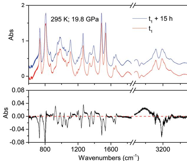
**Fig. 2** Difference spectrum (lower panel) obtained by subtracting the two spectra (upper panel) collected at ambient temperature and nearly the same pressure (19.8 GPa) 15 hours apart. Negative and broad positive peaks are related to disappearing and forming species, respectively.
