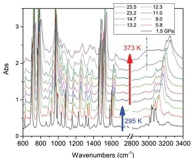
**Fig. 3** Evolution of the IR spectra of crystalline TS during a high temperature compression. The sample has been compressed at ambient temperature up to 9 GPa, heated at this pressure up to 373 K and then isothermally compressed. The reaction threshold has been identified at around 14 GPa. The broken line identifies the position of the broad C-H stretching band involving saturated carbon atoms.
