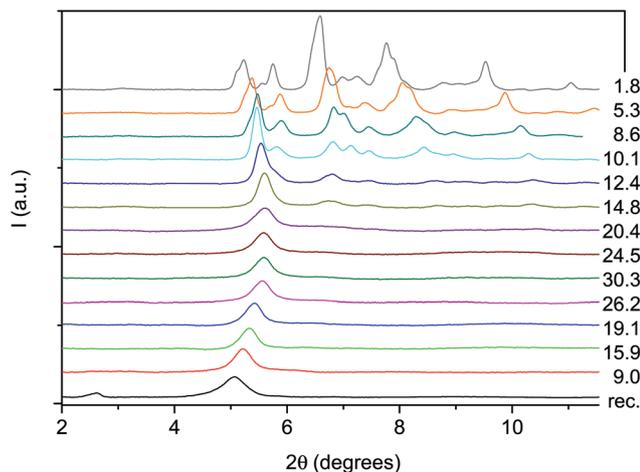
**Fig. 6** Selected X-ray diffraction patterns collected ( $\lambda = 0.49499 \text{ \AA}$ ) on pure TS during a room temperature compression–decompression cycle performed without pressure transmitting medium. The pressure values reported for each pattern are in GPa.
