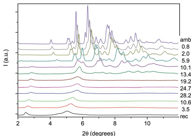
**Fig. 7** Selected X-ray diffraction integrated patterns collected ( $\lambda = 0.49499 \text{ \AA}$ ) for TS–TA mixed crystalline powder during a room temperature compression–decompression cycle performed without pressure transmitting medium. The pressure values reported for each pattern are in GPa.
