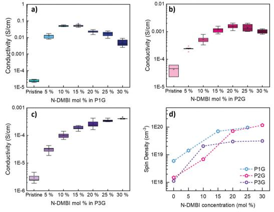
Fig. 2 σ of P1G (a), P2G (b), and P3G (c) films doped with N-DMBI. Representative I-V curves are shown in Fig. S7 (ESI†). (d) Shows a summary of the spin densities obtained from EPR
