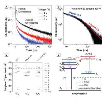
Fig. 5 (A) Transient EL decay of the non-doped device B2 at different voltages. (B) Amplified EL spectra of the non-doped device B2 at 5 V. (C) Energy diagrams. Energy levels and twice the T<sub>1</sub> energies (dashed line) of the anthracene derivatives calculated using B3LYP/6-311G(d,p), where nis the quantum number used to indicate the excited state. (D) Proposed TTU mechanism based on the emitters
