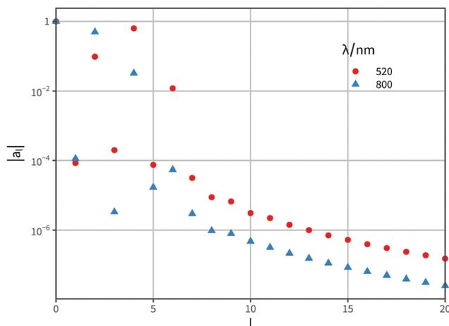
**Fig. 3** Spherical harmonic analysis of the circular dichroism angular patterns shown in Fig. 2(c). We use the function `sphharm` from the Matlab library `Chebfun`<sup>57,58</sup> to compute the decomposition of the angular map into spherical harmonics. For each harmonic degree  $l$  we collapse the
