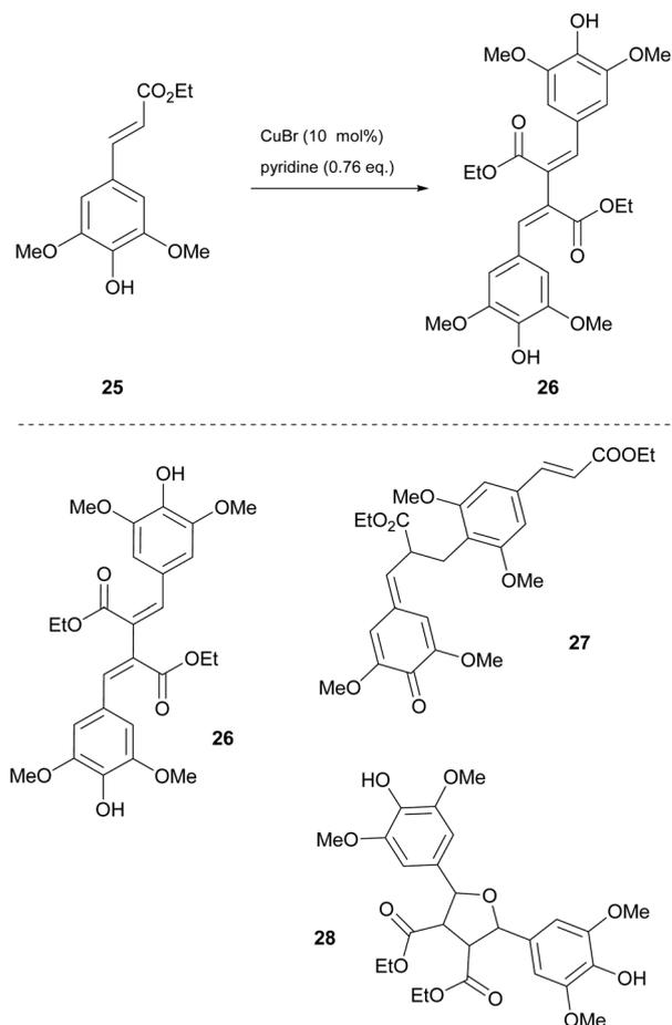
**Scheme 6** Synthesis of the sinapate β–β' dimer **26** using Cyrene as the solvent and various products of ethyl sinapate dimerization.
