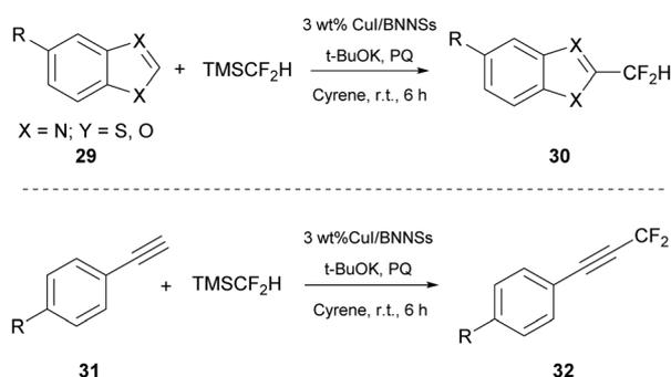
Scheme 7 Difluoromethylation of heteroarenes (**29**) and terminal alkynes (**31**) using Cyrene as the solvent. All reactions were performed with **29** or **31** (1.0 equiv.),  $\text{TMSCF}_2\text{H}$  (2.0 equiv.), catalyst (10 mg), *t*-BuOK (3 equiv.), and 9,10-phenanthroquinone (PQ) (1.2 equiv.).
