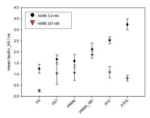
Fig. 4 Mean values with standard deviations of "\u03c4-Av\_Int", i.e., the average lifetime weighted on intensity, for MNP samples incubated with 170 nM HA-RB (red triangles) and 5.6 nM HA-RB (black circles).
