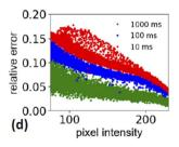
Fig. 4 Photographs of stable aerosol flow illuminated by a laser diode and recorded with different dwell times. (a) 10, (b) 100, (c) 1000 ms. The region surrounded by the green trapezoid symbolizes the region and direction of the sample flow (d) relative error for each pixel as function of pixel intensity, calculated from repeated images during a 30 second period.
