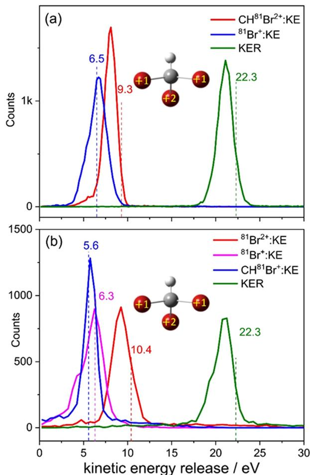
Fig. 12 Kinetic energy release distribution in three-body fragmentation of bromoform trication into (a) Br<sup>+</sup> + Br<sup>+</sup> + CHBr<sup>2+</sup> and (b) Br<sup>2+</sup> + Br<sup>+</sup> + CHBr<sup>+</sup>. The vertical dashed lines and numerical values are the results of our CES for concerted fragmentation with the charge distributions shown in the respective insets.
